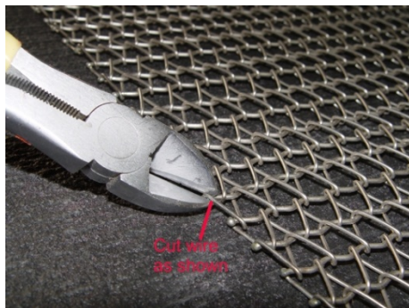
Making a Belt Splice Rod
