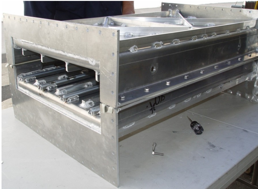
New Cooling Section with quartz rods
