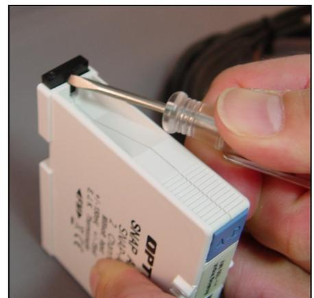
**Figure 7-18: I/O Module Removal**
