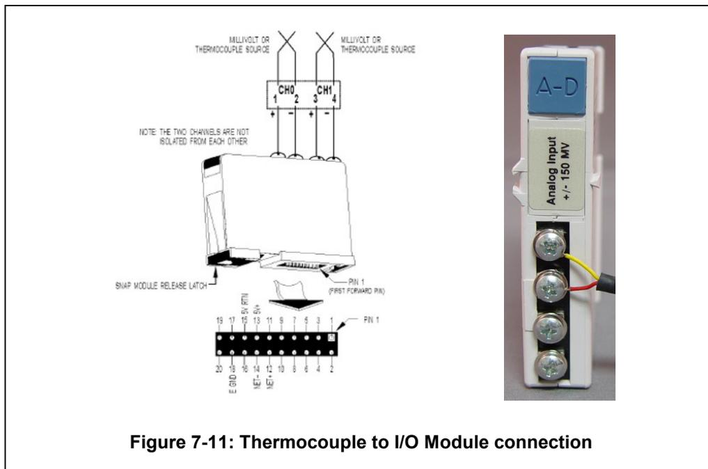
**Figure 7-11: Thermocouple to I/O Module connection**
