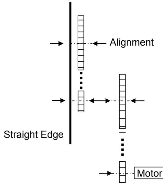
Figure 7-21: Sprocket Alignment
