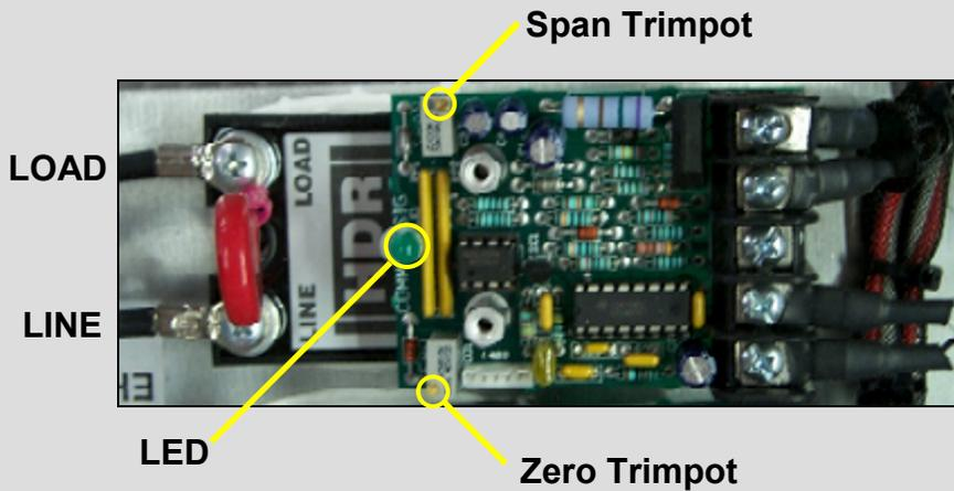
Figure 7-5: SCR Calibration Diagram & SCR Detail
