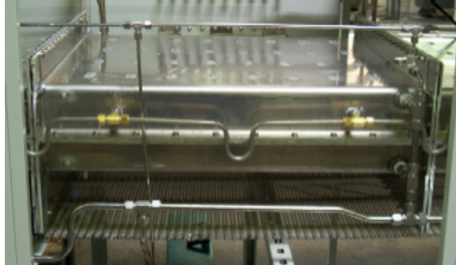
Figure 4-21: Water Cooled Controlled Atmosphere Cooling Module
