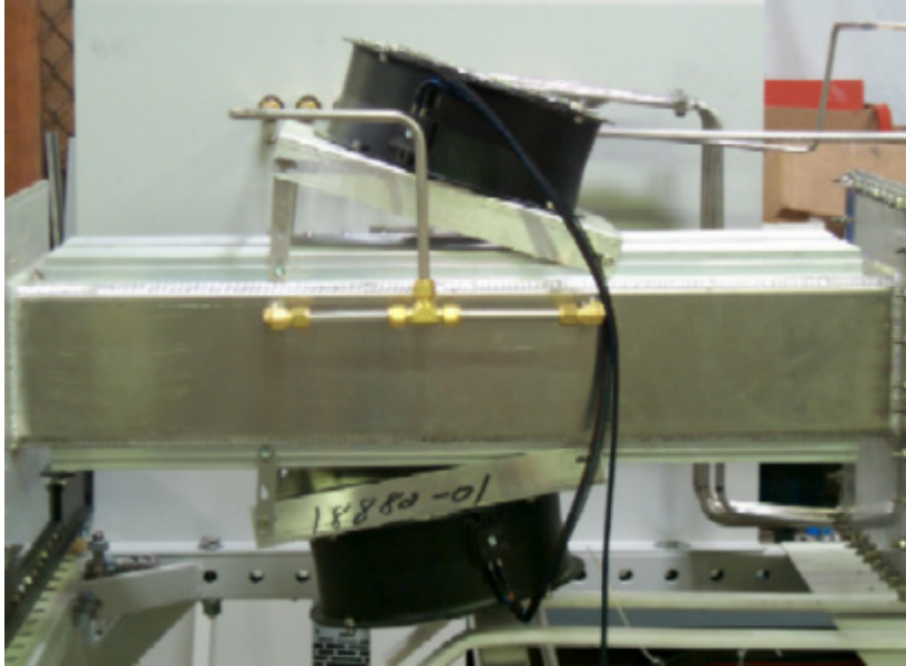
Figure 4-22: Controlled Atmosphere Air Cooled Module
