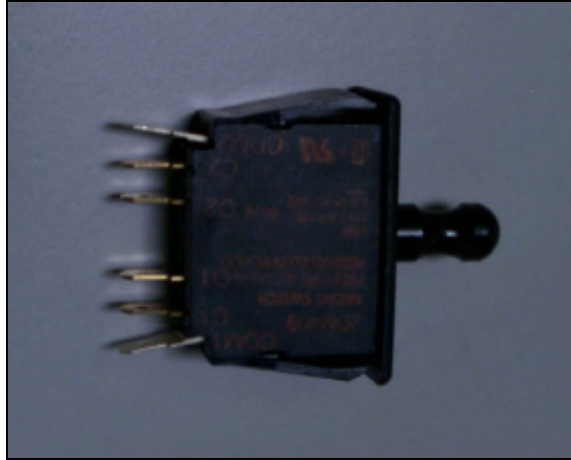
Figure 2-1: Panel Switches Showing Normal Operation Position
