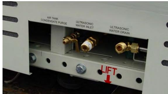
Figure 1-29 UCD Water Connections with Air Purge
