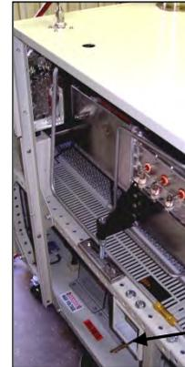
Figure 1-11 Typical Safety Interlock Disconnect Switch Location (option)
