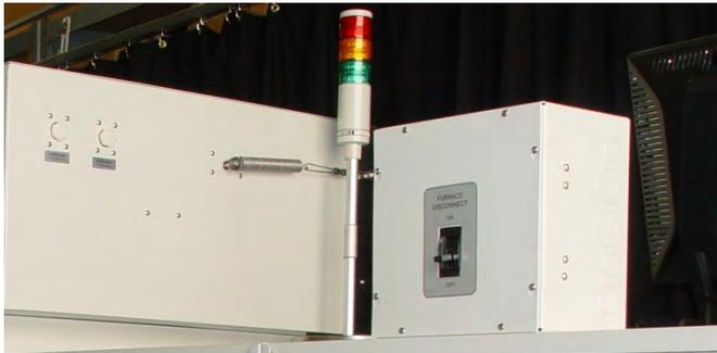
Figure 1-13 Typical Circuit Breaker Enclosure Location (option)
