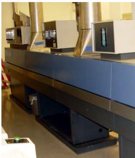
Figure 1-26 Cabinet Exhaust Example
