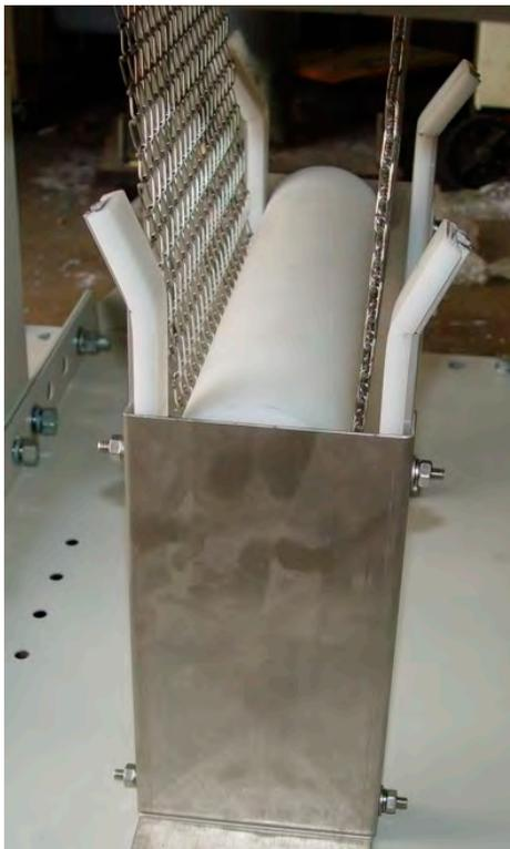
Figure 1-8 Belt Weight in Place
