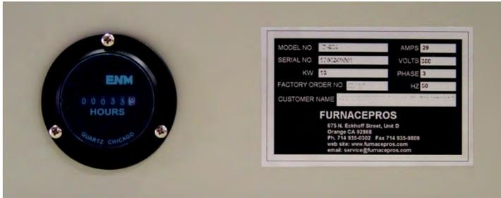
Figure 1-12 Elapsed Time Meter and Nameplate
