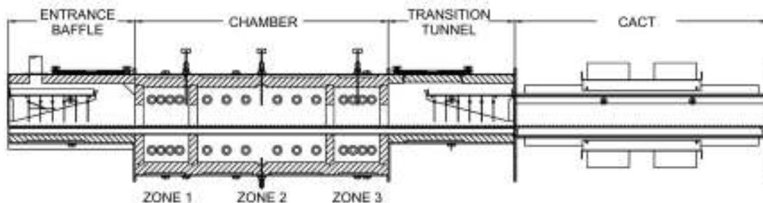
Figure 1-9 Furnace Internals
