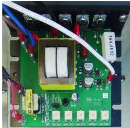
Figure 1-25 Motor Controller
