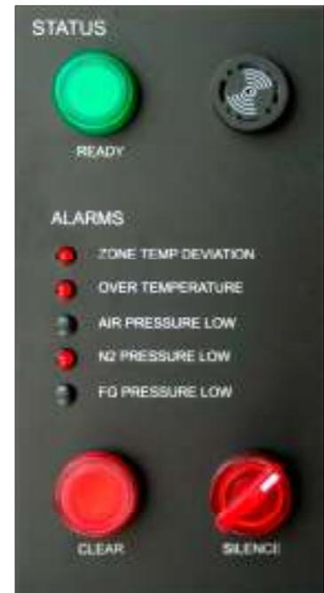
**Figure 1-19 Status Panel and Alarm Controls**
