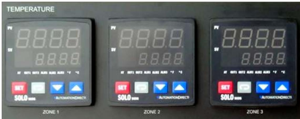
**Figure 1-13 Zone Temperature Controllers**
