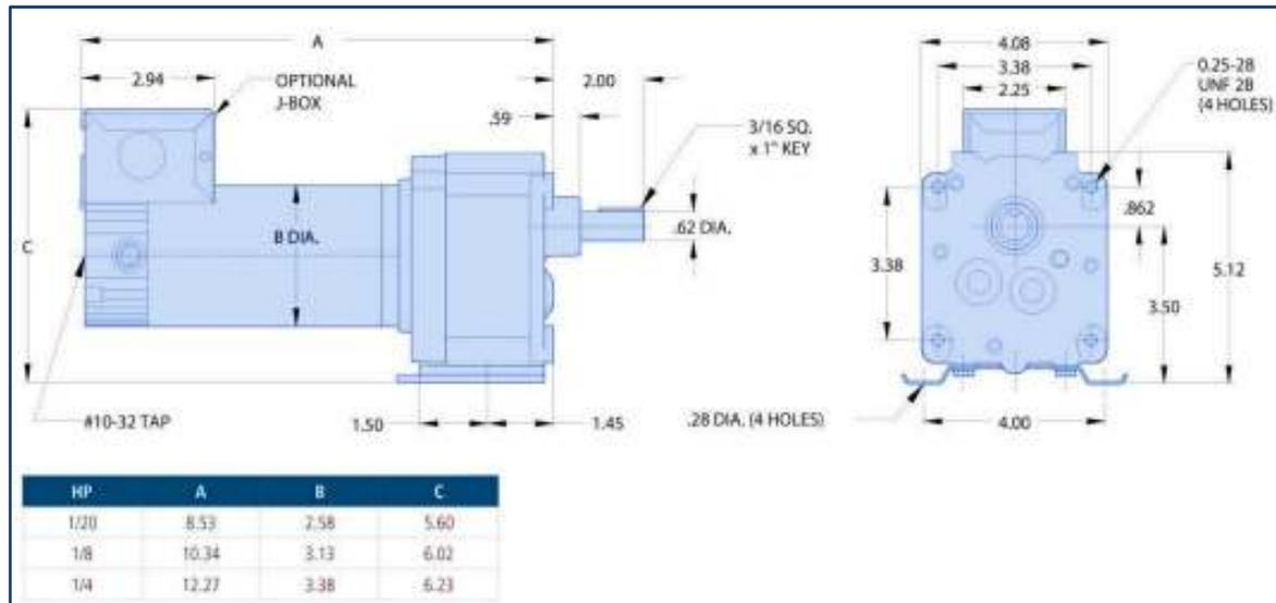
Figure 1-28 Transport Drive DC Motor
