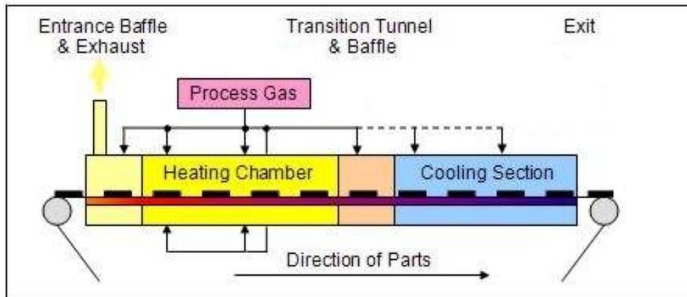
Figure 1-8 Process Sections
