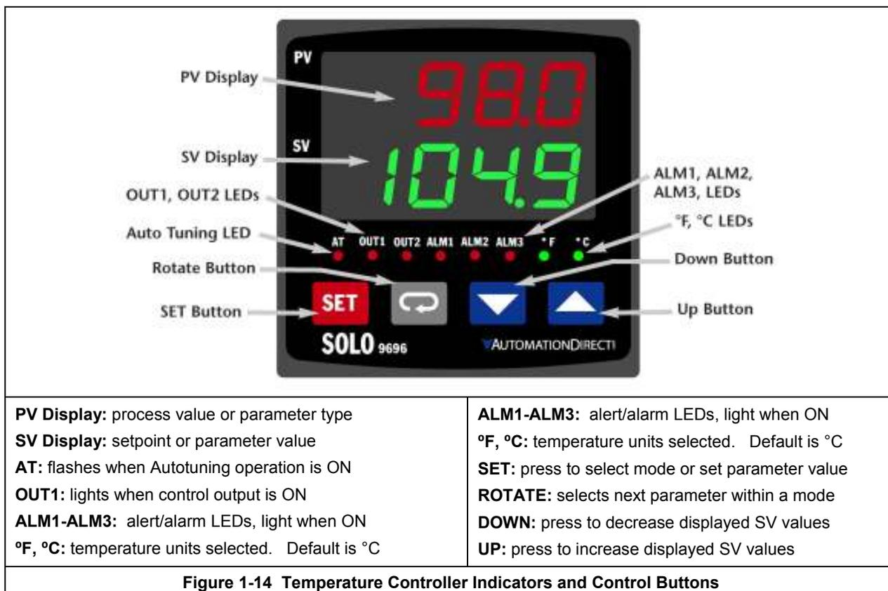
**Figure 1-14 Temperature Controller Indicators and Control Buttons**
