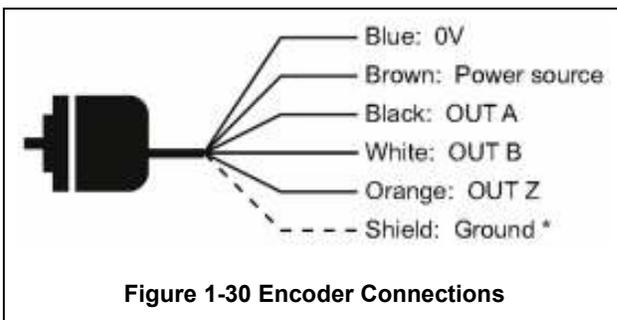
Figure 1-30 Encoder Connections
