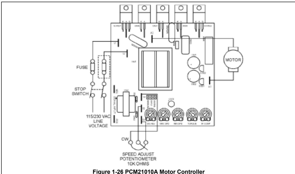
Figure 1-26 PCM21010A Motor Controller
