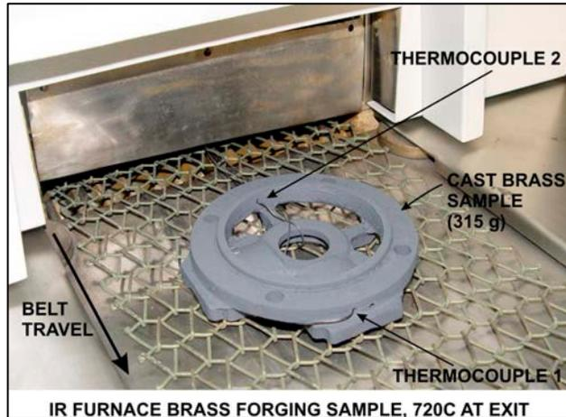
Figure 9-7 Brass Forging Sample With 2 thermocouples
