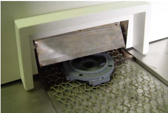
Figure 9-11 Brass forging sample exiting furnace
