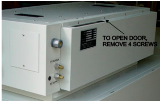
Figure 7-4 Control Enclosure Access Door Closed
