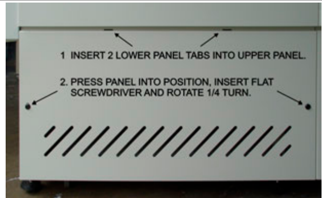
Figure 7-7 Lower Access Panel Installation
