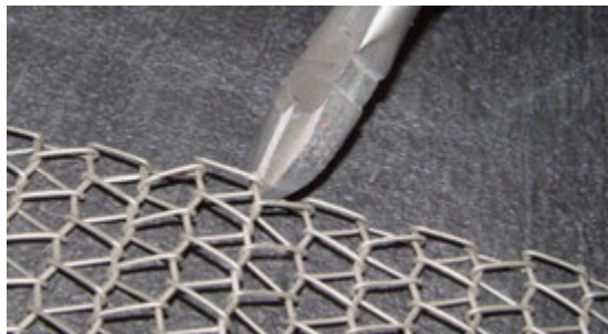
Figure 7-15 Second Cut at Opposite Side
