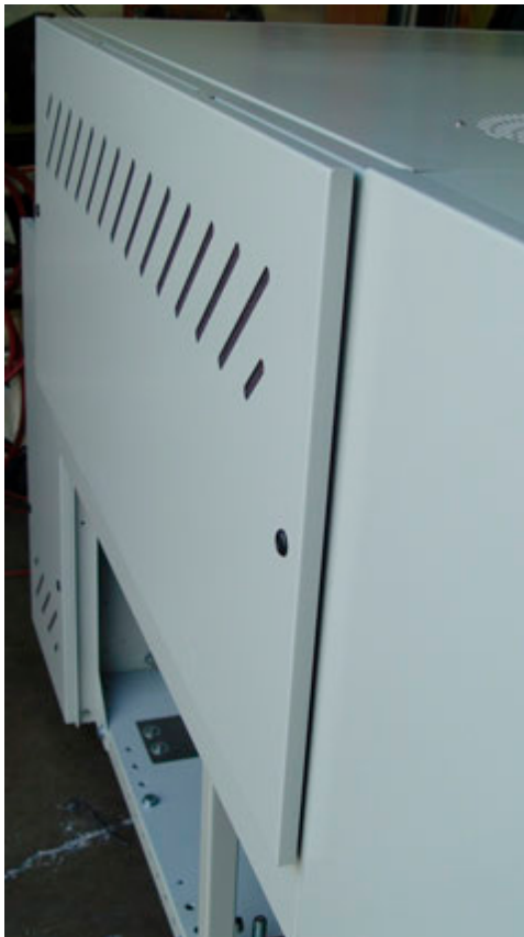
Figure 7-8 Hanging Lower Access Panel
