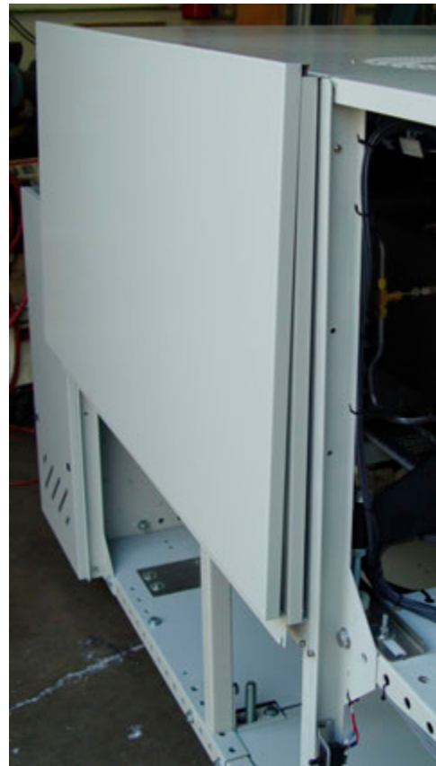
Figure 7-9 Hanging Lower Access Panel
