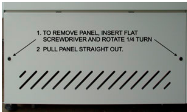
Figure 7-6 Lower Access Panel Removal
