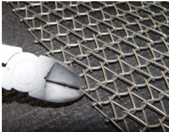
Figure 7-14 Cut Wire at Ball Joint
