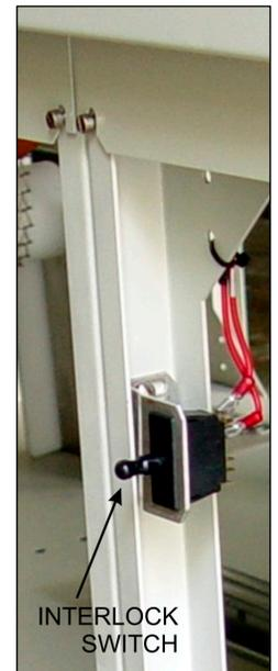
Figure 3-2 Lower Panel Interlock
