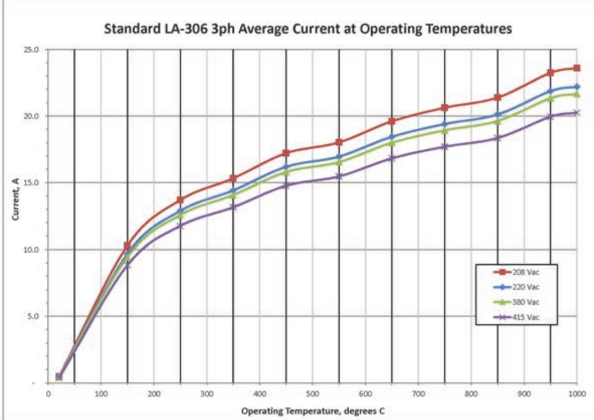
Expected three phase current draw when stabilized at various temperatures.
