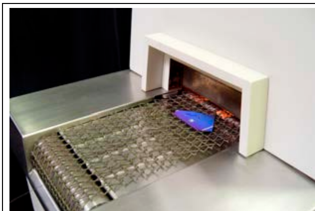
Figure 9-9 Silicon Wafer Entering Furnace
