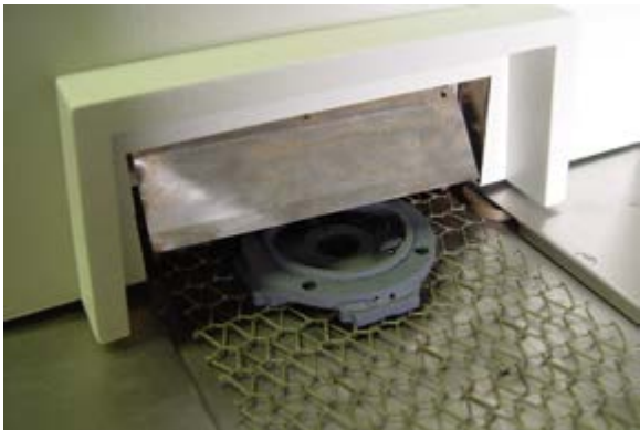
Figure 9-11 Brass forging sample exiting furnace
