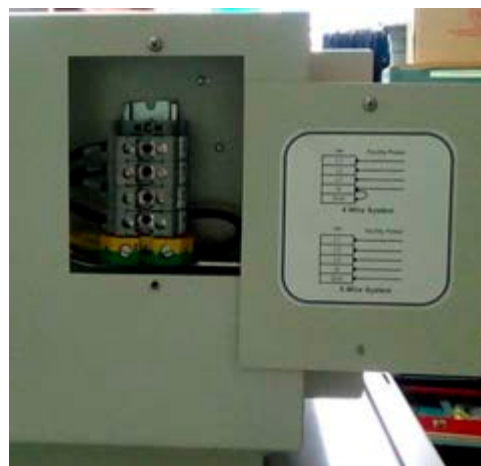
Figure 6-2 3-Phase Electrical (Option)
