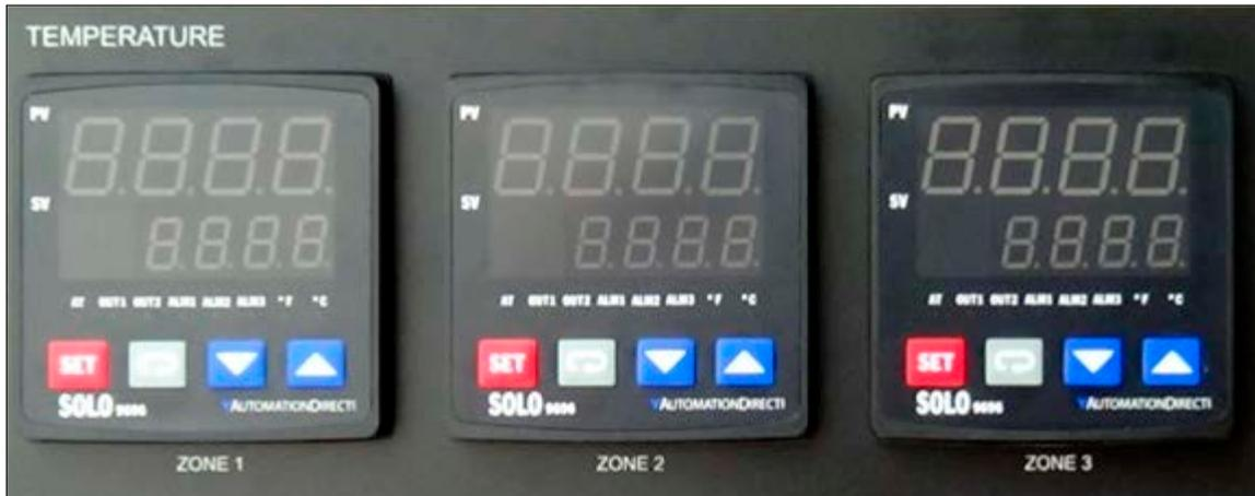
Figure 1-13 Zone Temperature Controllers
