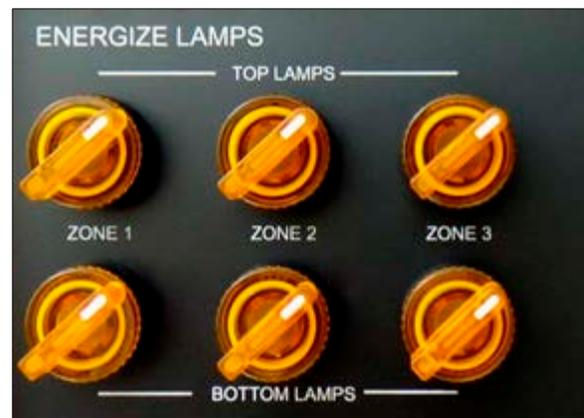
Figure 1-12 Energize Lamps control panel
