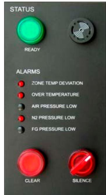
Figure 1-19 Status Panel and Alarm Controls
