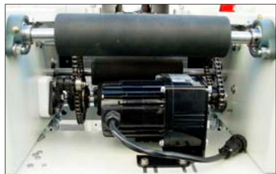
Figure 1-25 Transport Drive Motor
