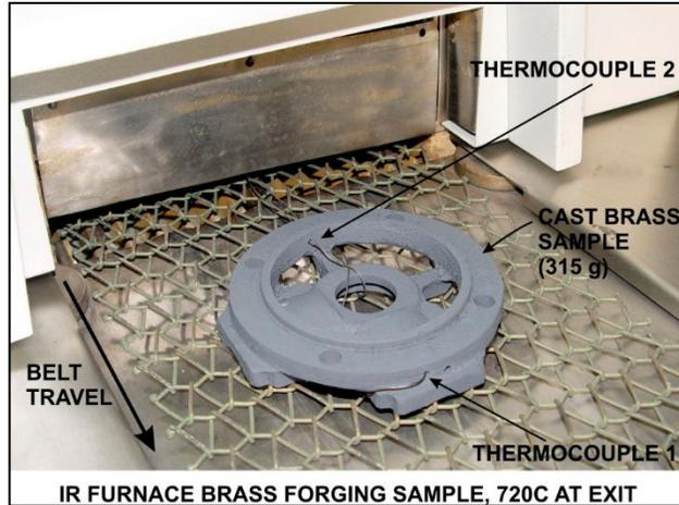
**Figure 6-7 Brass Forging Sample With 2 thermocouples**
