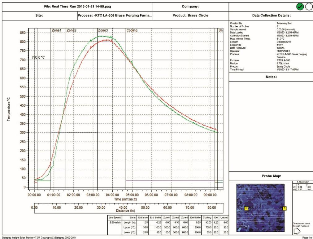
Figure 6-14 880 °C Brass Forging profile
