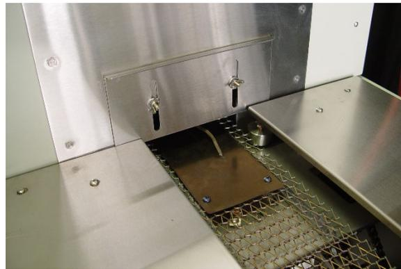
Figure 6-12 Sample plate exiting furnace
