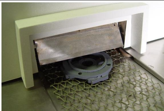
Figure 6-11 Brass forging sample exiting furnace
