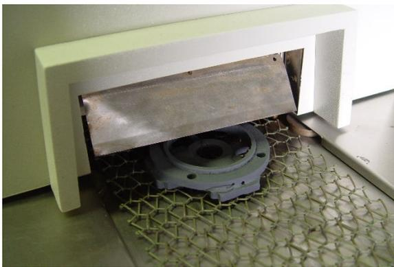
Figure 6-11 Brass forging sample exiting furnace
