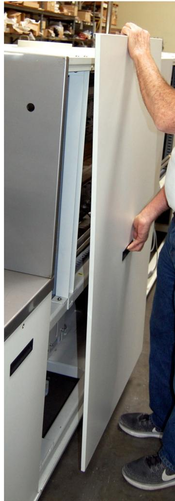
Figure 4-9 Lift panel straight up
