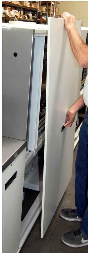
Figure 4-9 Lift panel straight up
