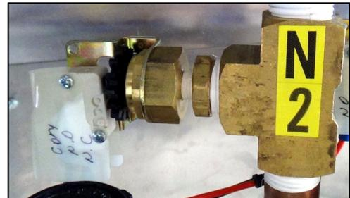
Figure 3-56 IPS Inlet Pressure Switch
