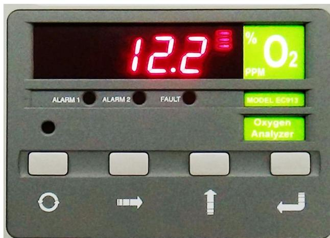
Figure 3-32 O<sub>2</sub> Analyzer Display
