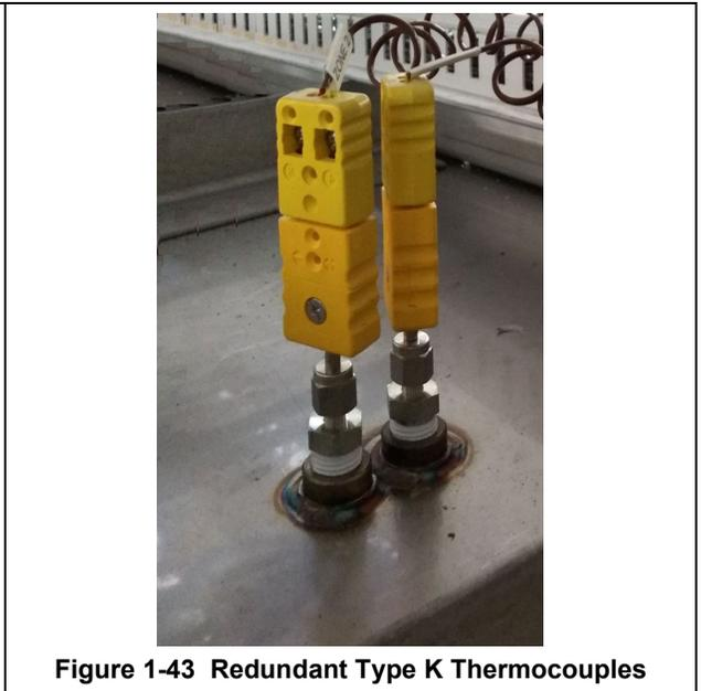
Figure 1-43 Redundant Type K Thermocouples
