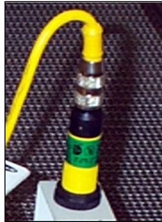
Figure 1-45 SMEMA Sensor closeup
