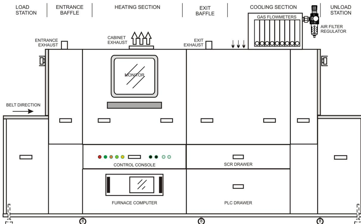
Figure 1-1 Furnace Front
