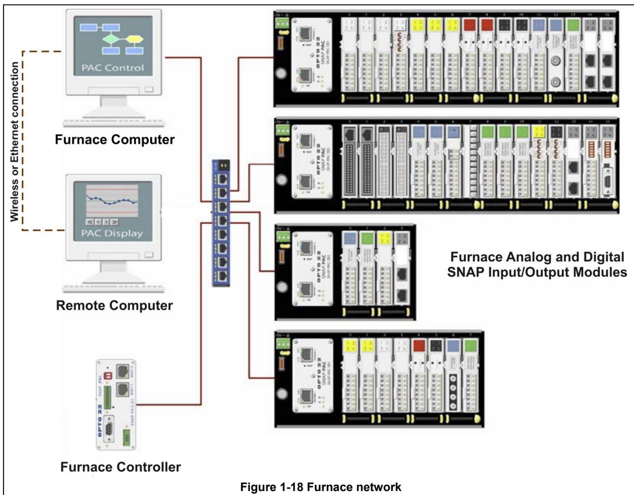
Figure 1-18 Furnace network
