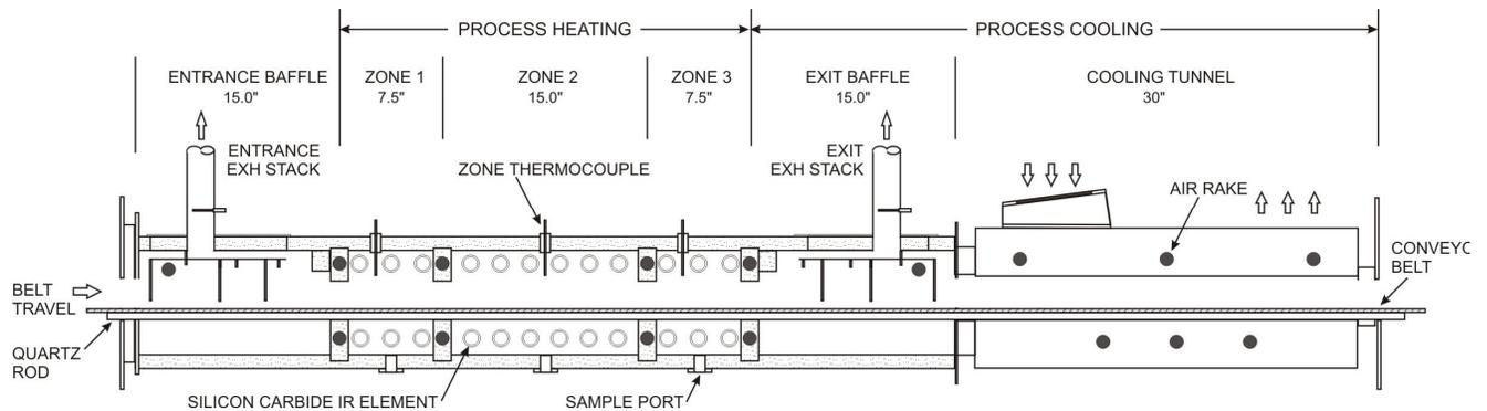
Figure 1-8 Furnace Internals
