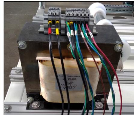
Figure 1-22 TR0 Main Transformer
