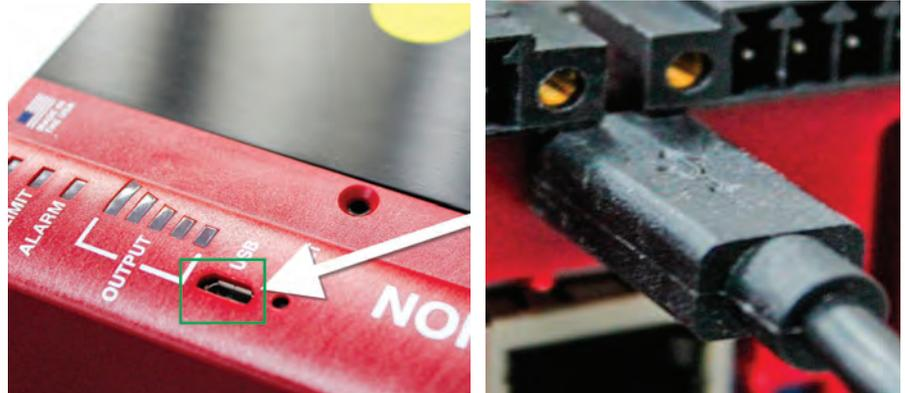
Figure 5.00: (Left) Location of the MicroUSB port of 1Ø Units; (Right) 3Ø Units have the MicroUSB port located between the P1 / P2 Connectors.
