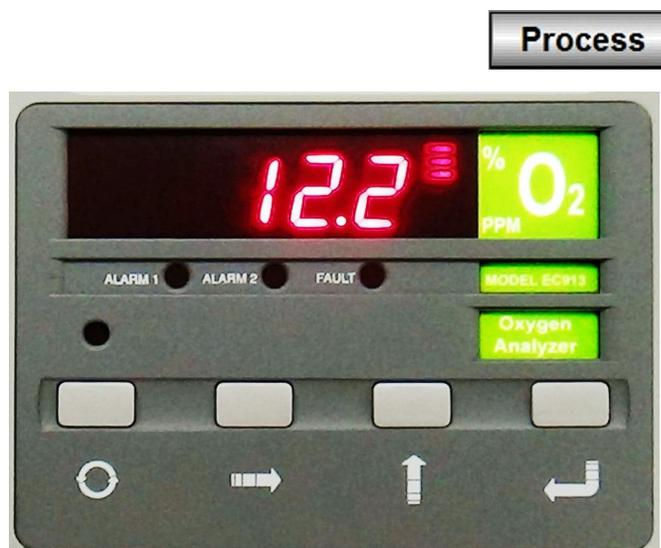
Figure 3-32 O<sub>2</sub> Analyzer Display
