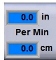
Figure 3-11 Belt Speed display
