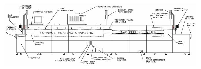
Figure 10.1.1 Typical Hydrogen Furnace
