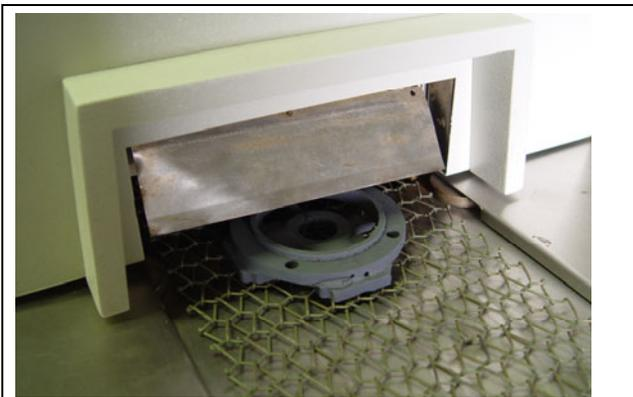
Figure 8-11 Brass forging sample exiting furnace
