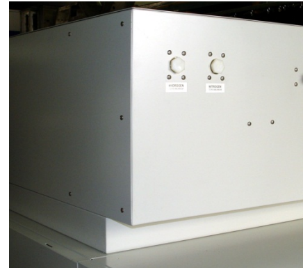
Figure 1-29 H2 & N2 Connections
