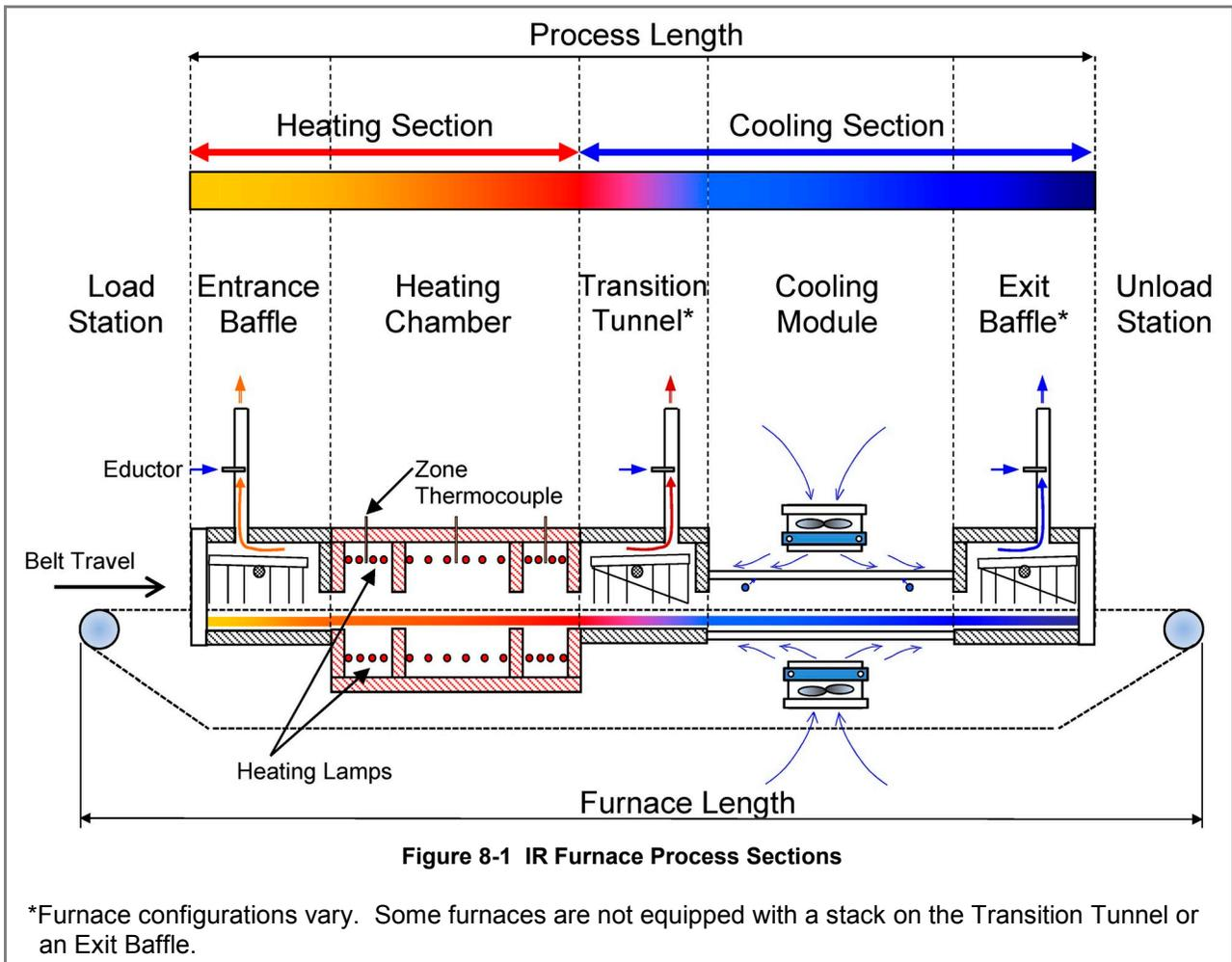
Continuous IR Processing is generally characterized by rapid ramping rates, ability to vary temperatures greatly from zone to zone and consistent processing performance in a controlled atmosphere. Establishing an acceptable profile and stabilizing the furnace are key to successful thermal processing. This is done by managing the following:
