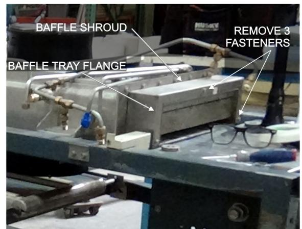
Figure 4-37 Exit Baffle Section Exposed
