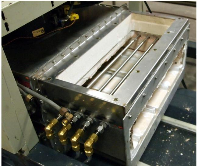
Figure 4-43 Transition Tunnel, Baffle Tray removed
