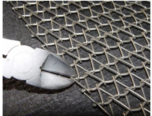
Figure 4-22 Cut wire at ball joint
