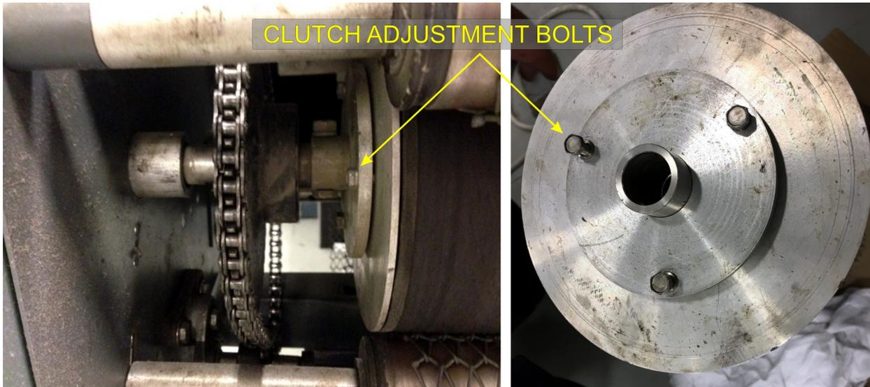
Figure 4-19 Clutch Adjustment
