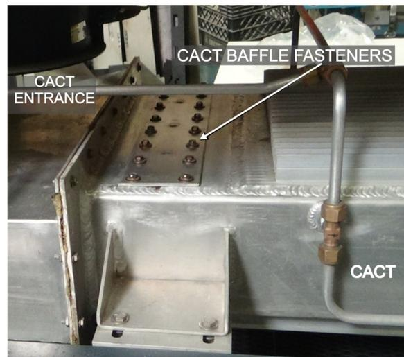
Figure 4-45 CACT Baffle fasteners
