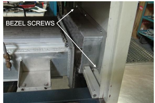
Figure 4-35 Bezel fasteners
