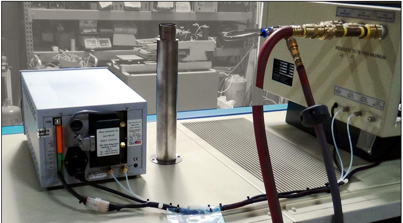
Figure 4-12 Oxygen Analyzer furnace connections
