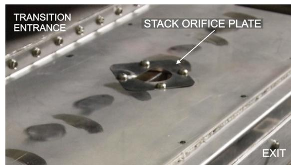
Figure 4-40 Transition Tunnel Stack Orifice Plate
