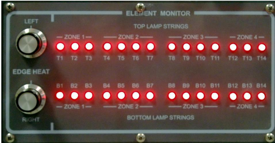
**Figure 4-17 Test Panel: Lamp String Failure Indicator**
