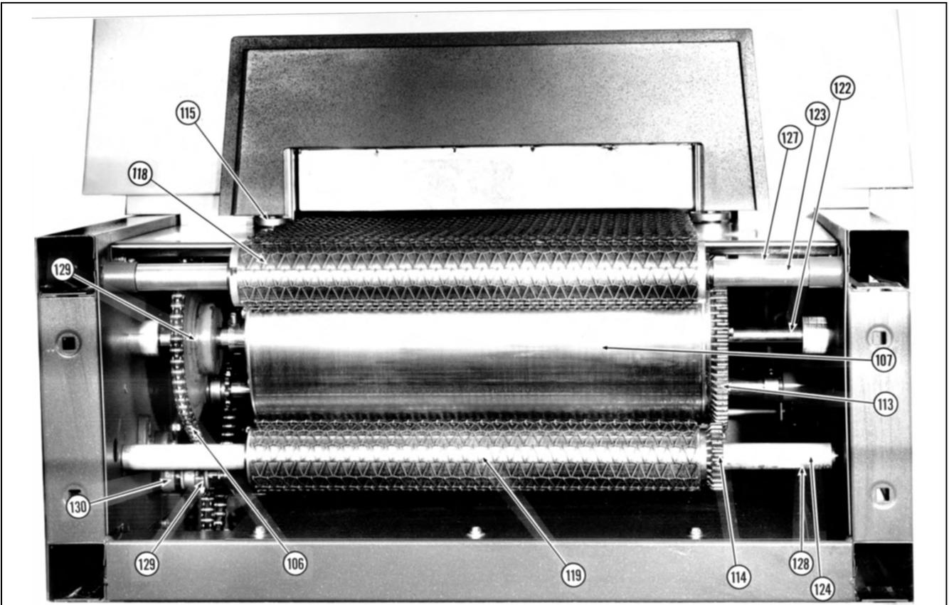
Figure 4-16 Transport Drive at exit
