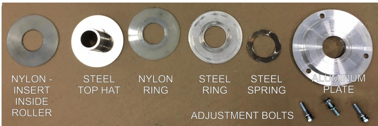
Figure 4-20 Clutch Components
