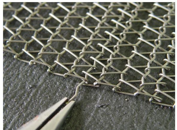
Figure 4-24 Remove belt wire
