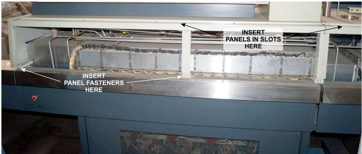
Figure 4-4 Upper Access Panel Installation
