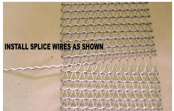
Figure 4-25 Insert splice wire
