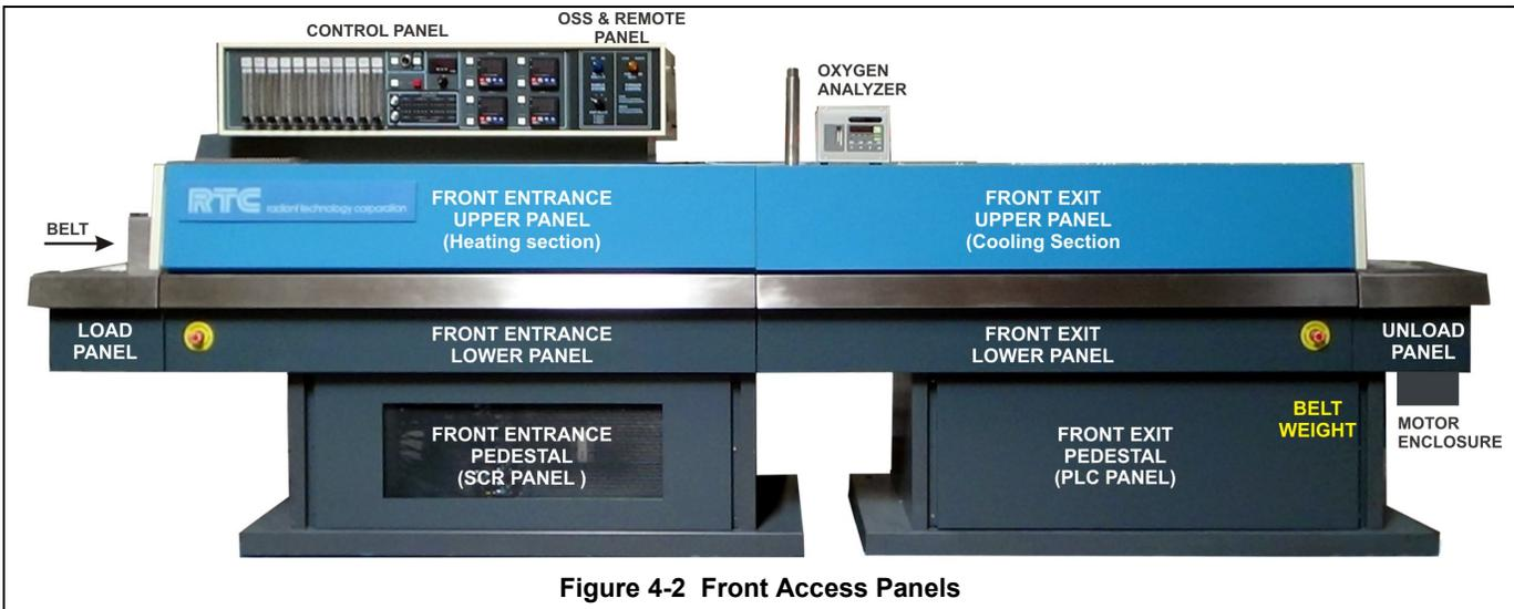
**LOWER PANELS.** To remove a Lower Panel: After the corresponding Upper Panel has been removed, lift the lower panel and pull toward you. Lower panels provide access to lower lamps, sample ports and/or bottom of cooling section.
