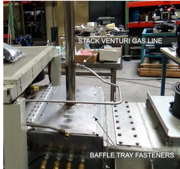
Figure 4-38 Transition Tunnel
