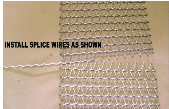
Figure 4-28 Align belt sections
