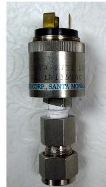
Figure 4-54 Gas Pressure sensor
