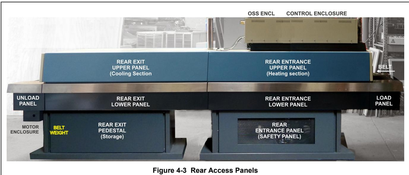
**COOLING SYSTEM.** Remove Front and/or Rear Exit Upper and Lower panels to access cooling system.
