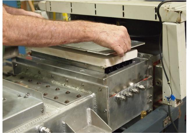
Figure 4-41 Baffle Tray in Transition Tunnel
