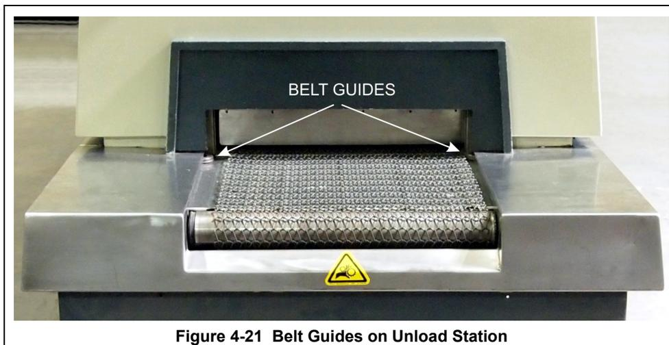
Figure 4-21 Belt Guides on Unload Station
