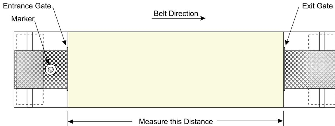
Figure 4-52 Belt Speed Calibration Diagram
