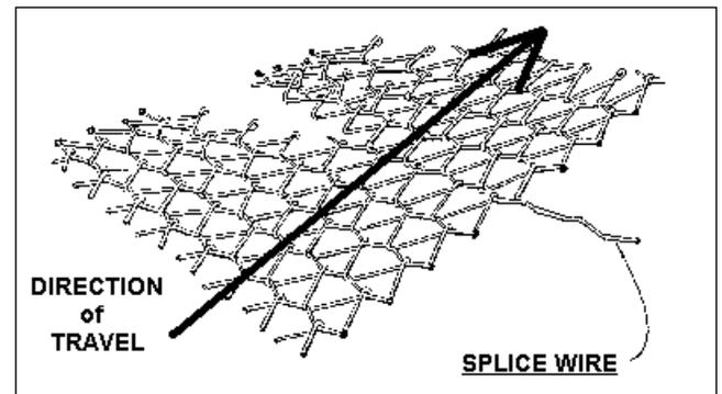
Figure 4-29 Insert splice wire
