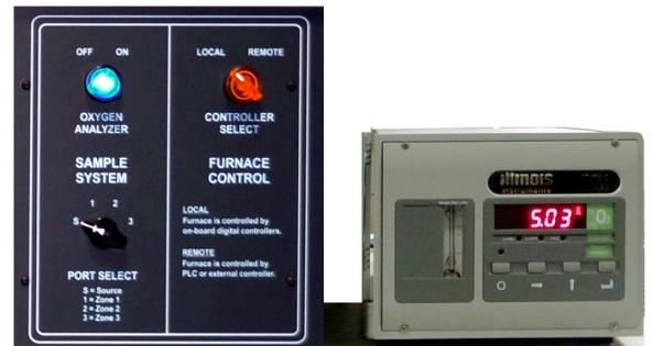
Figure 3-2 Sample System Console & Oxygen Analyzer ON
