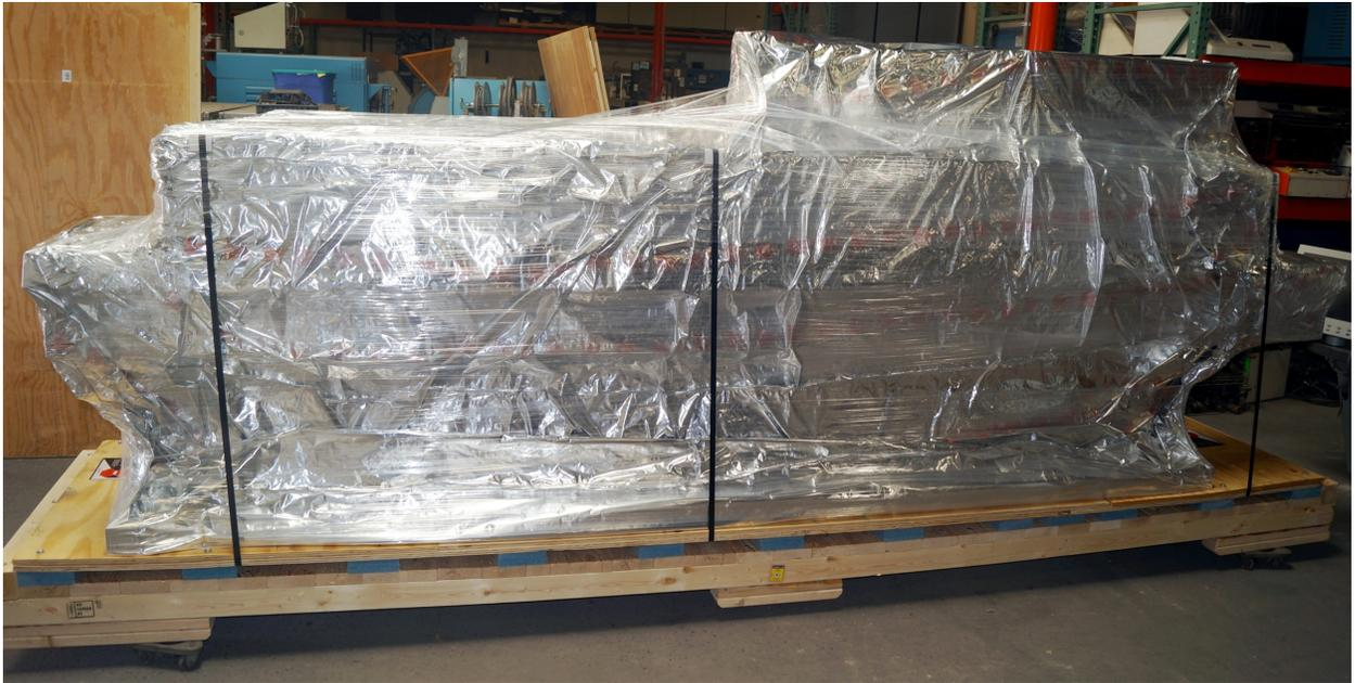
Figure 2-1 Furnace banded to Pallet Skid with Moisture Protection
