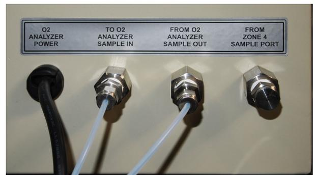
Figure 2-41 OA furnace control enclosure connections
