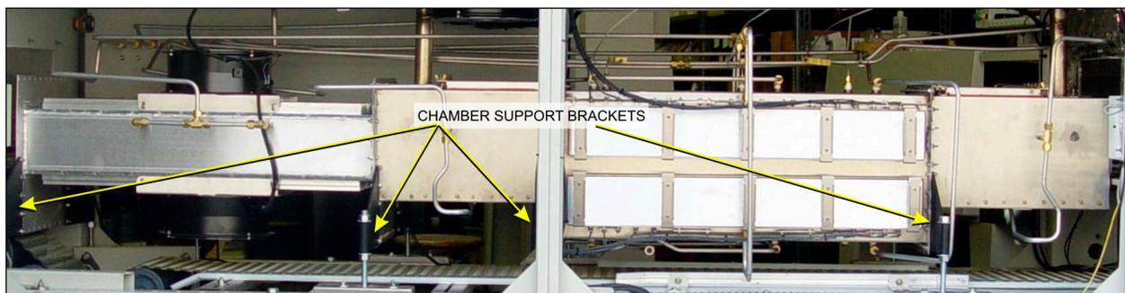
Figure 2-13 Location of Support Brackets on post-2000 model furnaces
