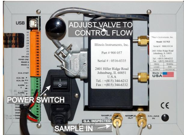
Figure 2-42 EC913 Oxygen Analyzer Rear Controls
