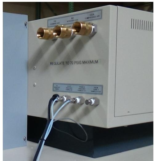
Figure 2-28 Process Gas Supply location
