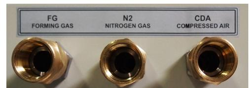
Figure 2-30 3-Process Gas connections
