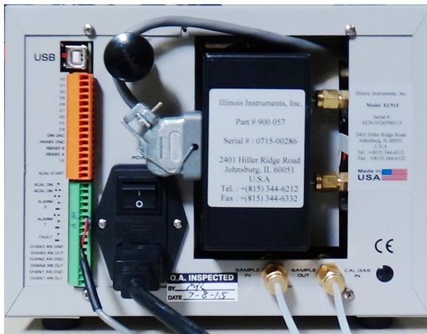
Figure 2-40 Oxygen Analyzer connections
