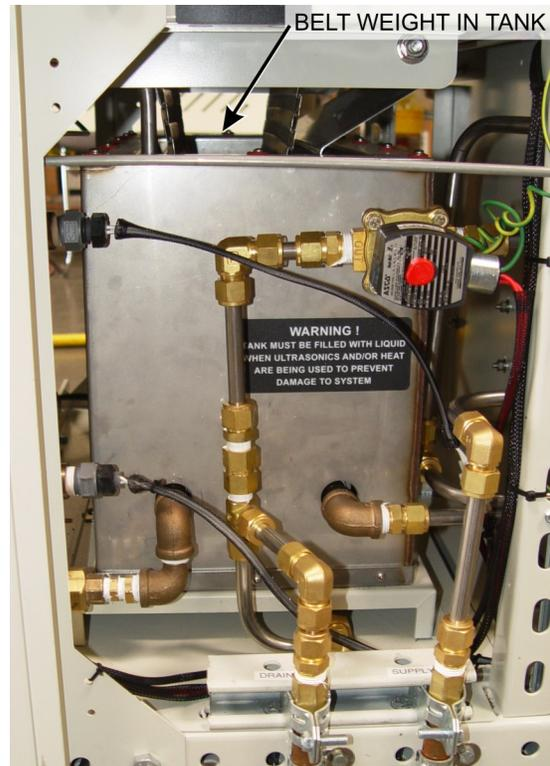
Figure 2-22 Belt weight in Tank on UCD system
