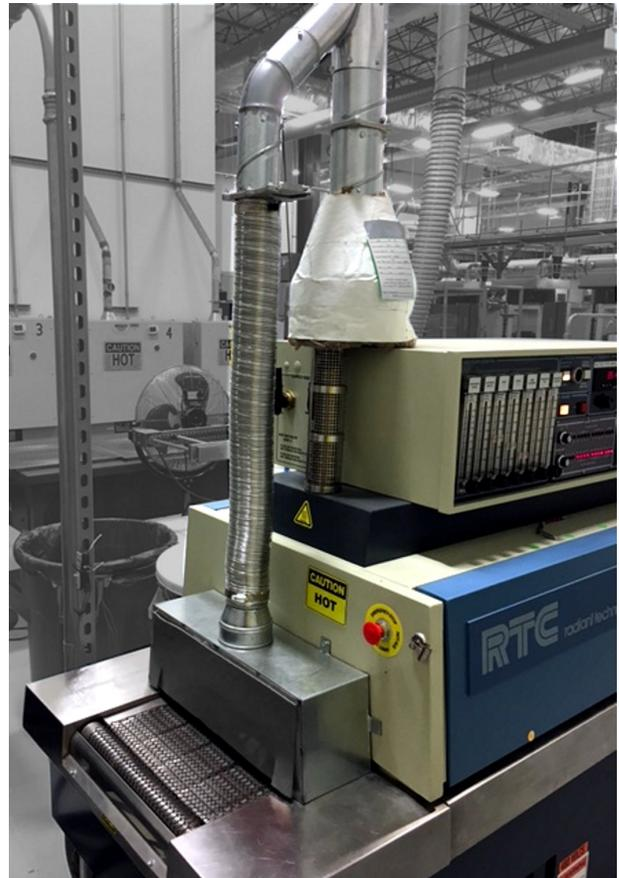
Figure 2-34 Collector Hood Exhaust Example
