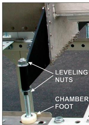
Figure 2-11 Chamber Support Bracket
