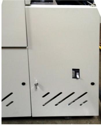
Figure 2-25 Circuit Breaker panel
