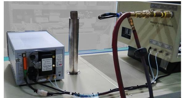
Figure 2-39 Locate oxygen analyzer next to OSS
