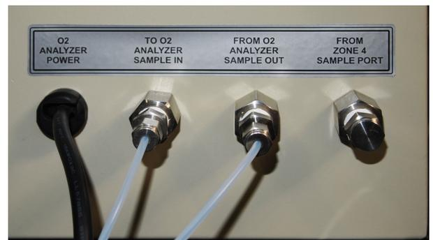
Figure 2-41 OA furnace control enclosure connections
