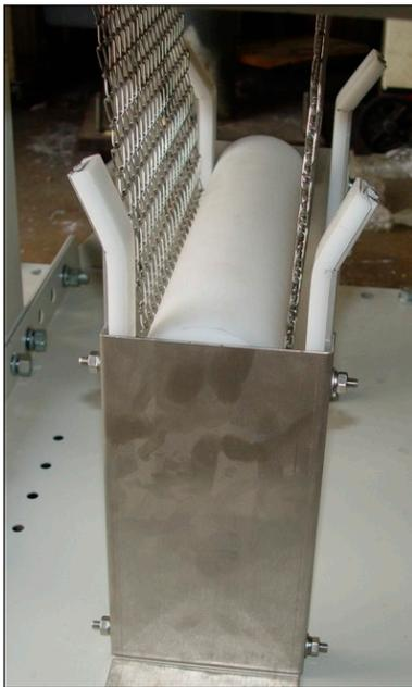
Figure 2-18 Belt Weight in guide
