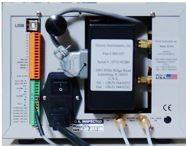
Figure 2-40 Oxygen Analyzer connections
