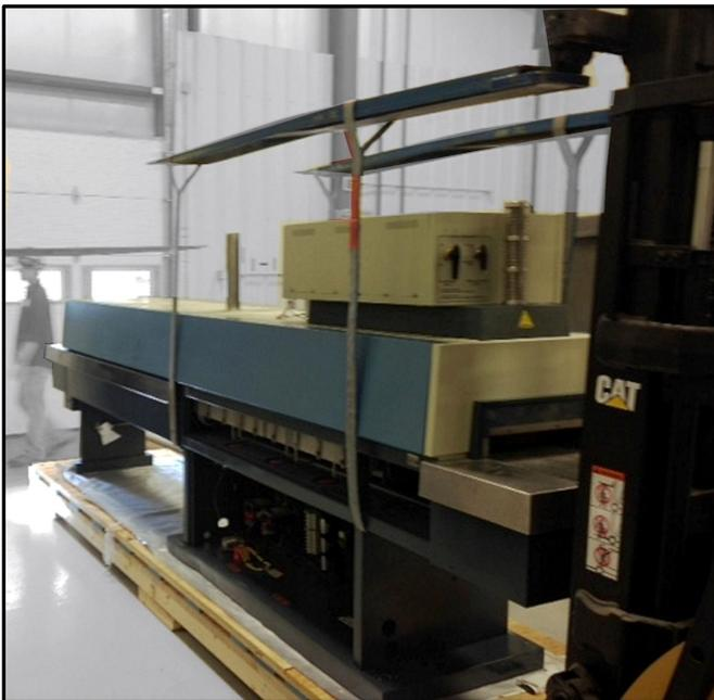
Figure 2-4 Lift Furnace with panel removed. Two-pedestal models may require the middle lift point closer to exit.
