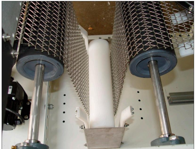
Figure 2-19 Proper Alignment of Belt Weight in guide
