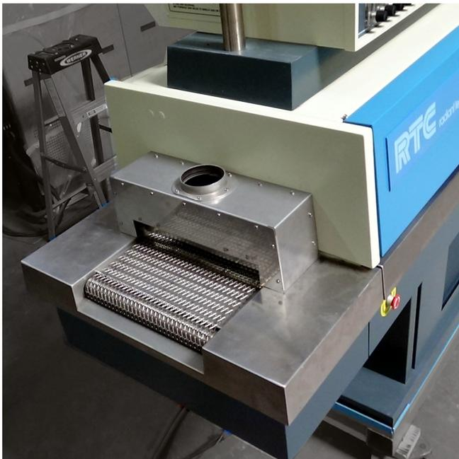
Figure 2-33 Collector Hood with baffle
