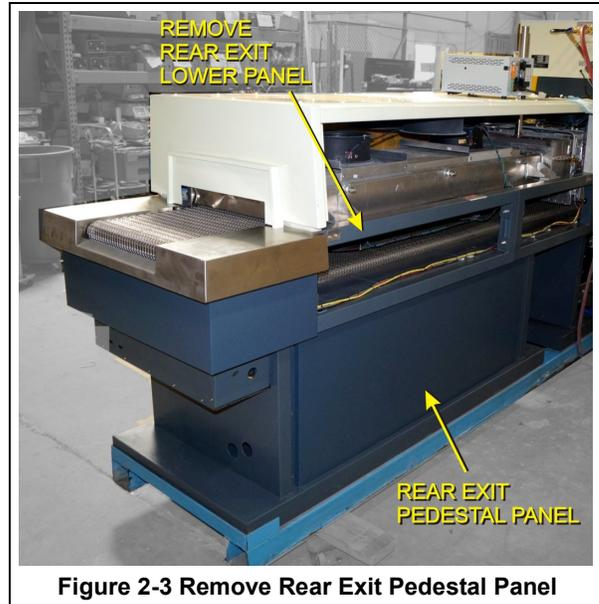
Figure 2-3 Remove Rear Exit Pedestal Panel
