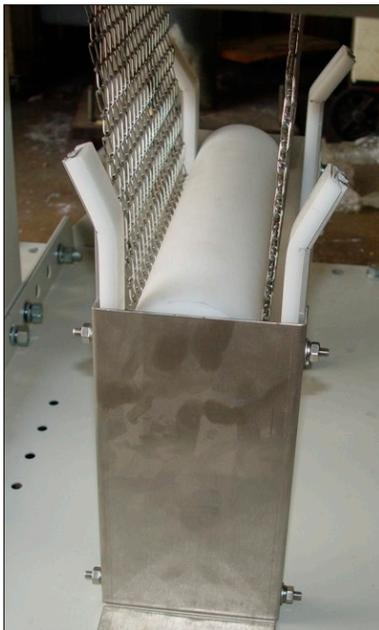
Figure 2-18 Belt Weight in guide
