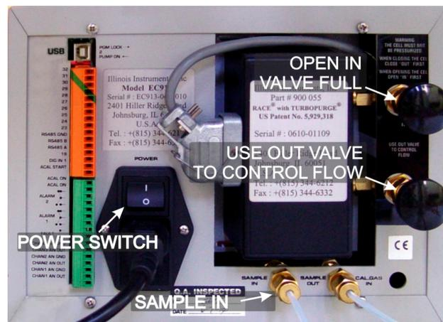
Figure 0-30 Oxygen analyzer next to OSS sample system
