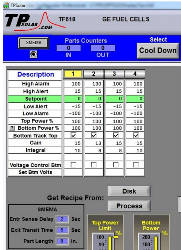
Figure 0-35 Screen showing Product Tracking settings
