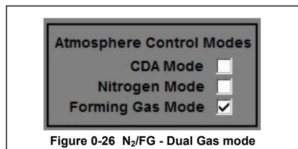
The furnace will operate with nitrogen flowing to the Aux furnace sections and Gas 2, forming gas or other alternate supplied gas flowing to furnace and lamp plenums.
