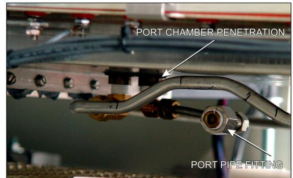
**Figure 0-36 Sample Port Chamber Penetration**
