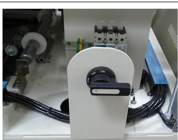
Figure0-22 3-Phase Circuit Breaker-Panel OFF
