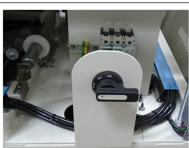
Figure0-22 3-Phase Circuit Breaker-Panel OFF
