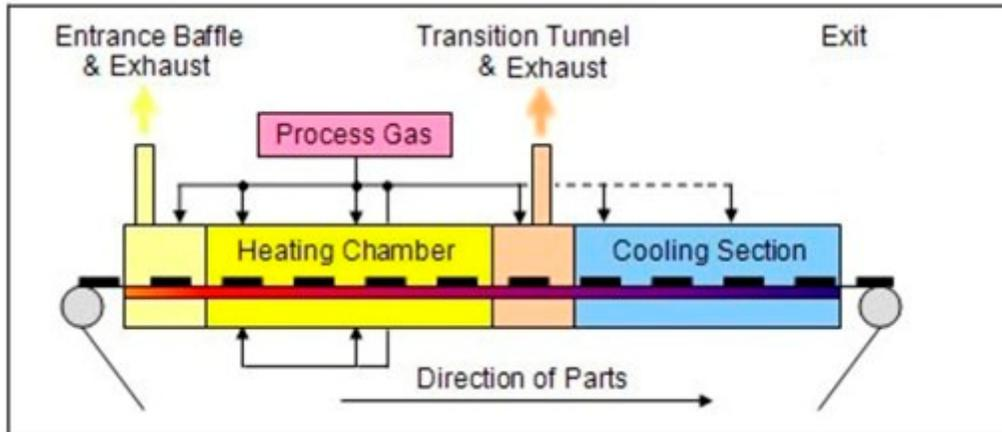
Figure 0-7 Process Sections
