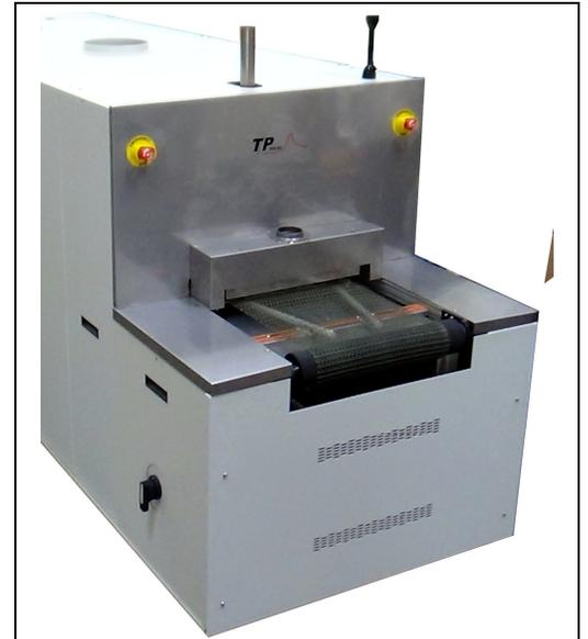
Figure 0-23 LA-309 Unload station with 600
