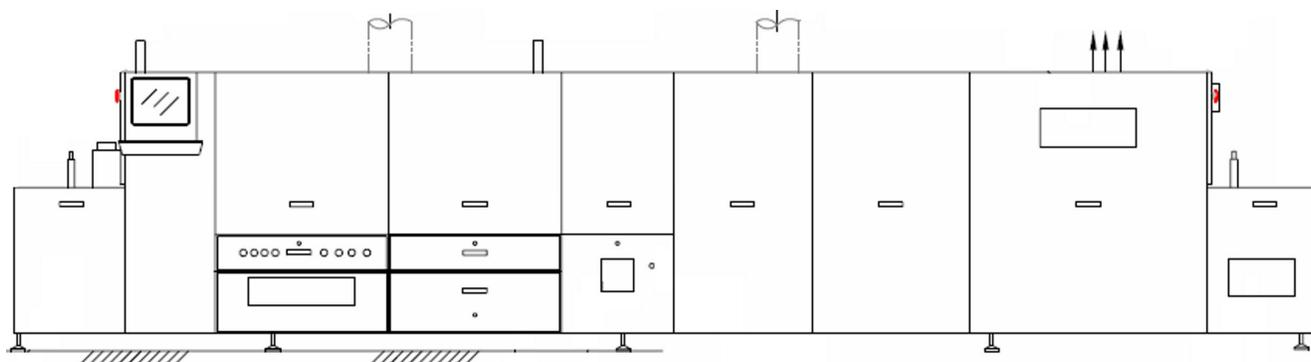
**Figure 0-1 TF-618 IR Furnace Front Elevation**
