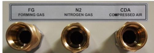
Figure 2-24 3-Process Gas connections
