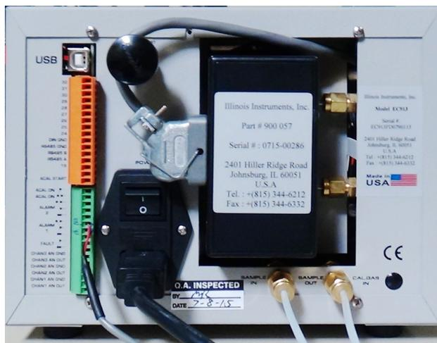
Figure 2-32 Oxygen Analyzer connections
