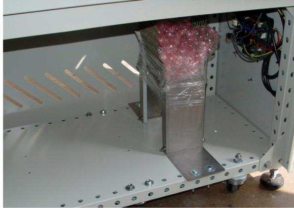
Figure 2-11 Belt Weight in guide with packing
