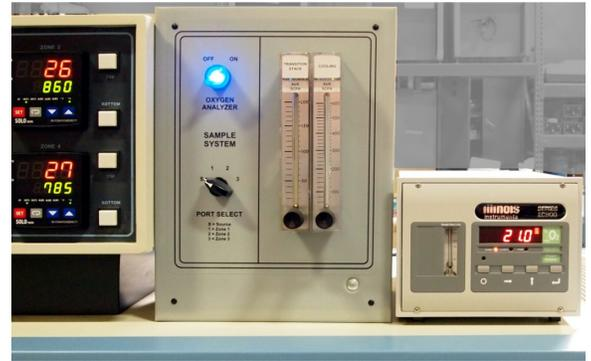
Figure 2-30 Oxygen analyzer next to OSS system
