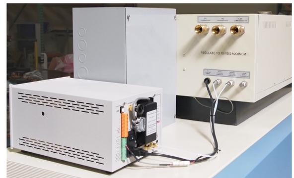
Figure 2-31 Locate oxygen analyzer next to OSS
