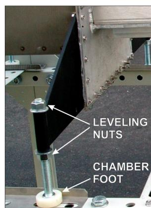
Figure 2-5 Chamber Support Bracket
