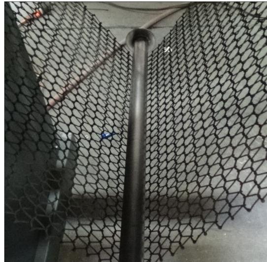
Figure 2-15 Proper Alignment of Belt Weight
