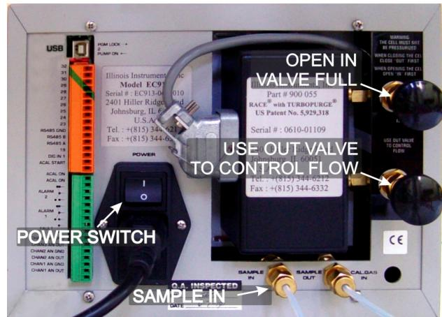
Figure 2-34 EC913 Oxygen Analyzer Rear Controls
