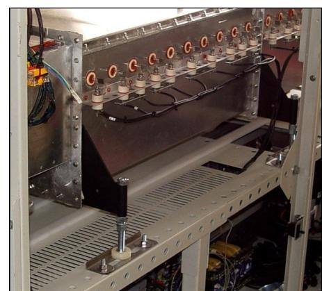
Figure 2-6 Chamber Support Brackets
