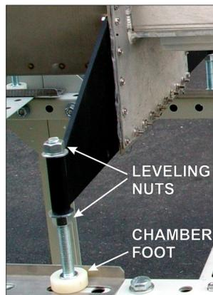
Figure 2-5 Chamber Support Bracket
