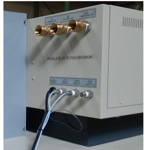
Figure 2-22 Process Gas Supply location
