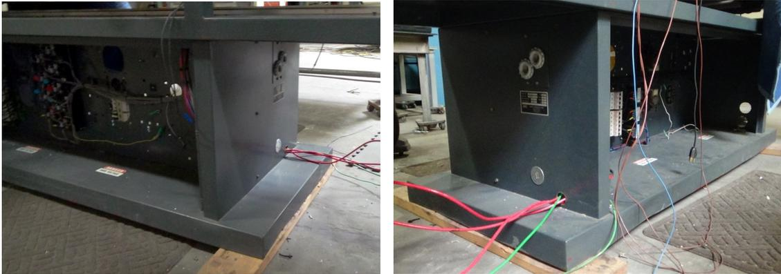
**Figure 2-17 Facility Power Port and Nameplate**
