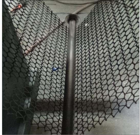
Figure 2-15 Proper Alignment of Belt Weight
