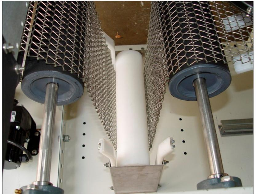
Figure 2-13 Proper Alignment of Belt Weight in guide
