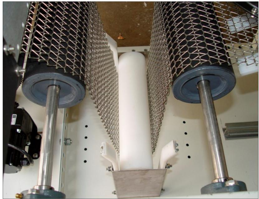
Figure 2-13 Proper Alignment of Belt Weight in guide
