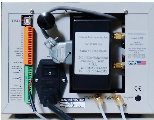
Figure 2-32 Oxygen Analyzer connections
