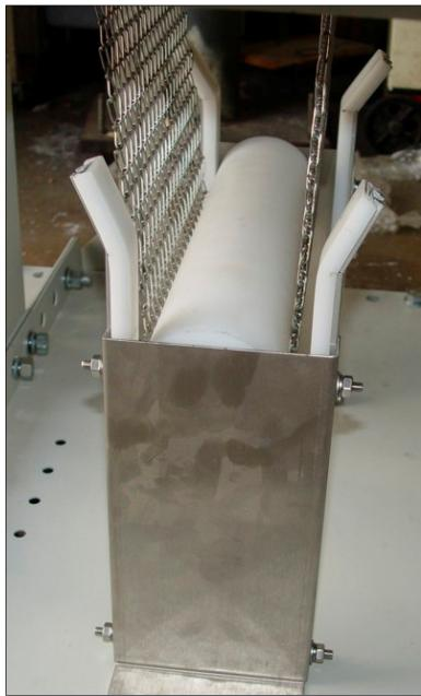
Figure 2-12 Belt Weight in guide
