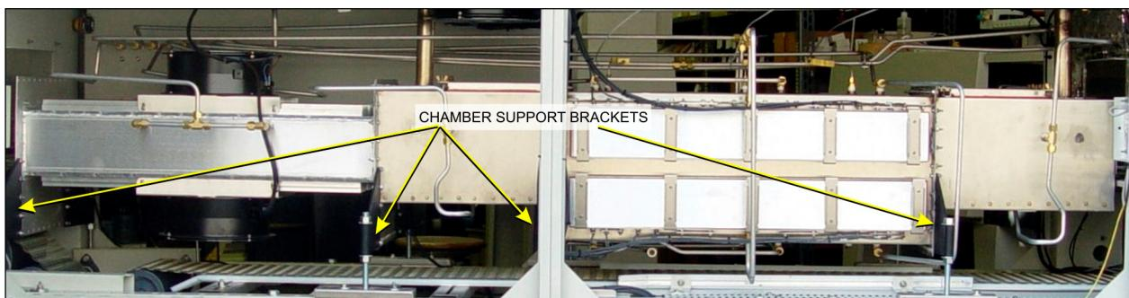
Figure 2-7 Location of Support Brackets on post-2000 model furnaces
