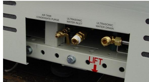
Figure 2-35 UCD Water Connections and Air Purge (Reservoir option only)
