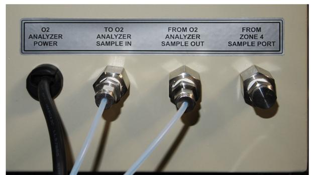
Figure 2-33 OA furnace control enclosure connections
