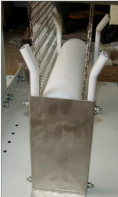
Figure 2-12 Belt Weight in guide
