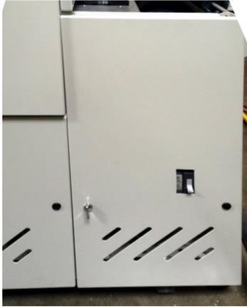
Figure 2-19 Circuit Breaker panel
