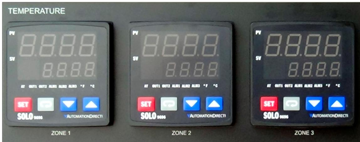
Figure 1-18 Zone Temperature Controllers
