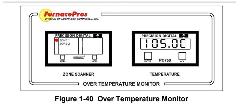
The OT system is in addition to the standard high/low temperature Alert/Alarm system included with the furnace controllers and/or software.
