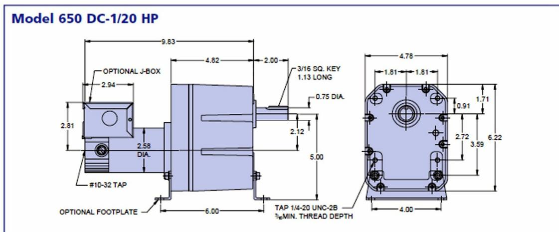
Figure 1-25 DC Drive Motor, Low Speed
