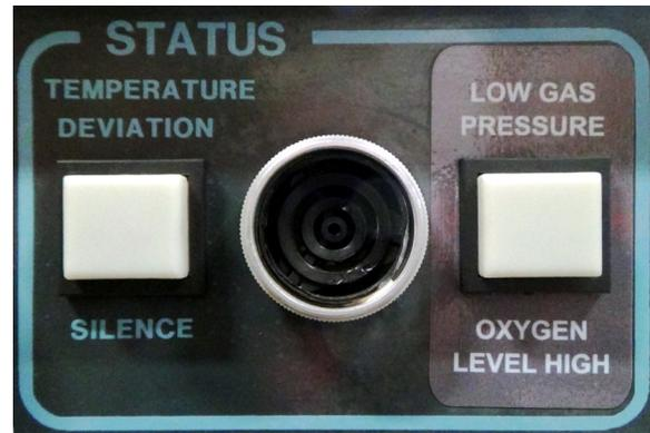
Figure 1-12 Status Panel and Alarm Controls
