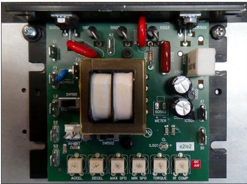
Figure 1-20 Motor Controller
