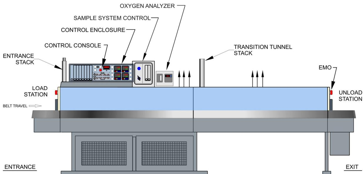
Figure 1-1 CU-915 IR Furnace Front Elevation
