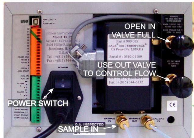
**Figure 1-39** EC913 Oxygen Analyzer Rear Controls
