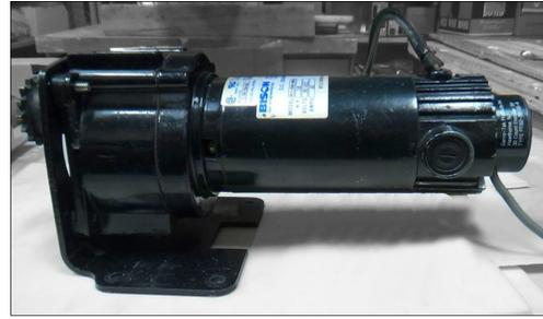
Figure 1-22 Drive Motor, Medium Speed
