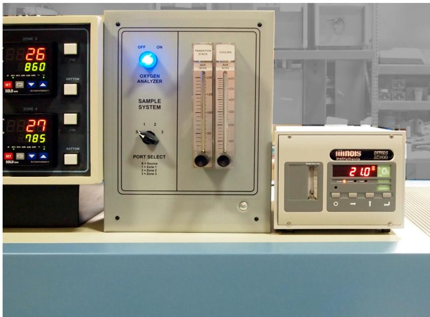
Figure 1-37 Oxygen analyzer next to OSS sample system
