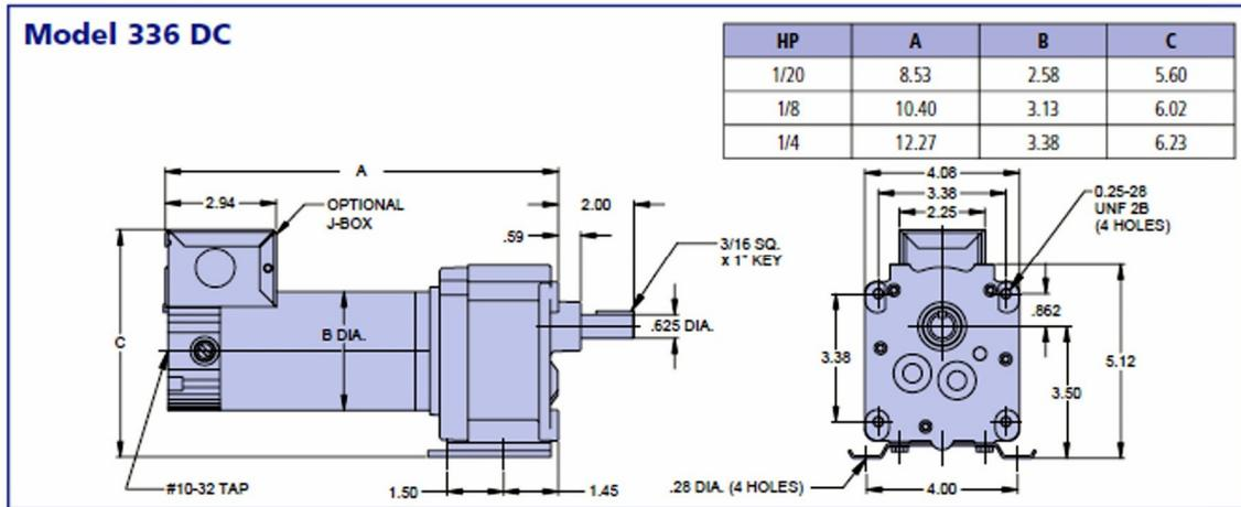
Figure 1-23 DC Drive Motor, Medium Speed
