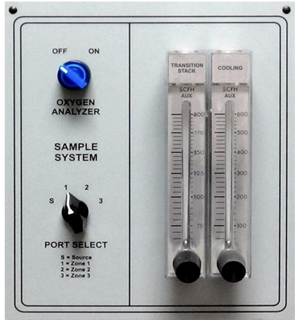
**Figure 1-38** Sample System control panel (shown with 2 Aux Flowmeters)
