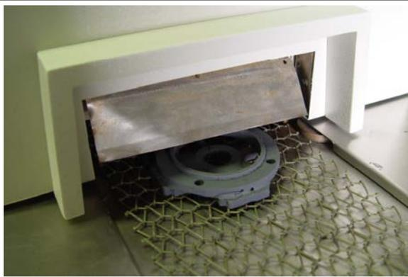
Figure 9-11 Brass forging sample exiting furnace
