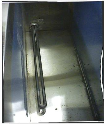
**Immersion Heater Bars Extend Into Tank to Heat Fluids**
