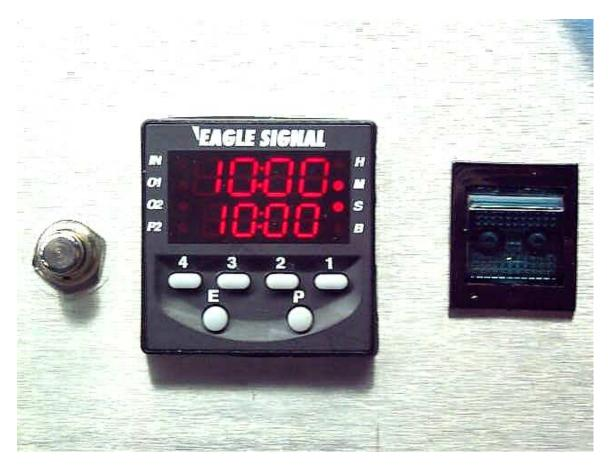
The digital timer is a black device that will be mounted to the control panel, and will have a digital backlit LED display. The large red on top of the smaller numerals in the center of the display represents the timer current value, while the smaller numerals at the bottom of the display represents the current set-point of the timer.
