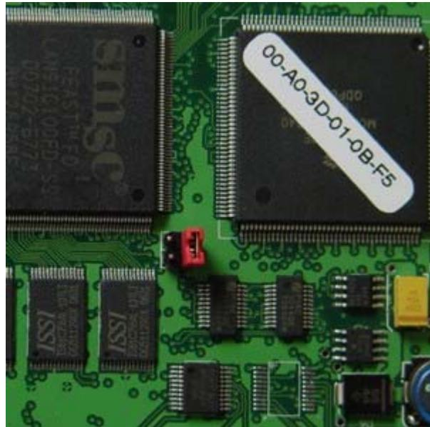
Figure 3.16.6 Move J7 Jumper to Module Reset
