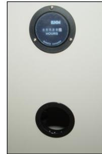
Figure 1.2.4 Power Port and Elapsed Time Meter
