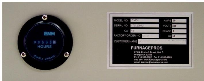
Figure 1.2.6 Elapsed Time Meter and Nameplate
