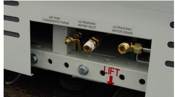
Figure 1.2.13 Water Connections and Air Purge
