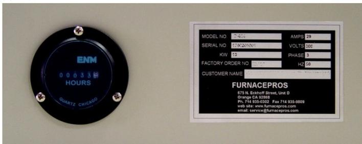
Figure 1.2.6 Elapsed Time Meter and Nameplate
