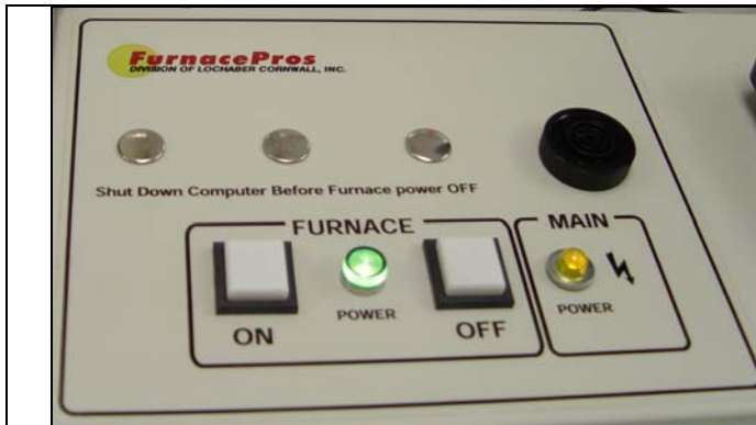
Figure 2.1.1 Control Panel showing Furnace Power ON and OFF and Indicator Lights
