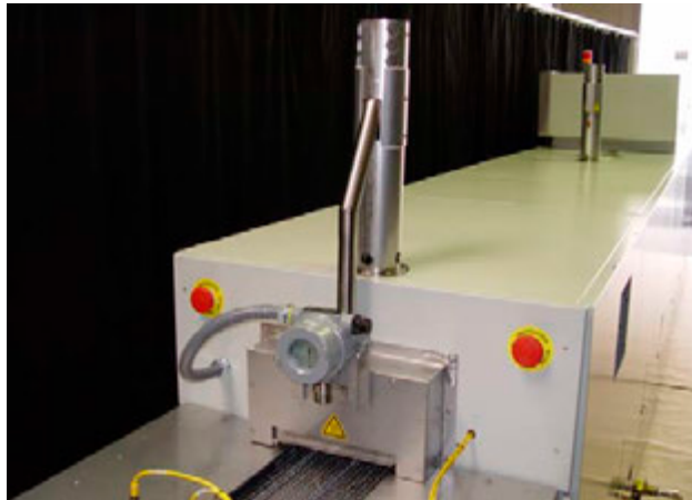
Exit showing Combustion Gas sensor, Collector & Igniters
