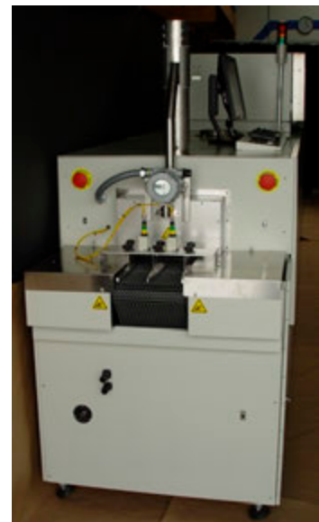
S-1209XH Entrance showing Hydrogen Sensor, SHEMA Product Sensors and Ignitor
