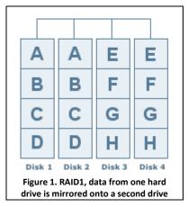
As shown in Figure 1, in a RAID 1 array, data from one hard drive is mirrored onto a second hard drive, so that there are two identical copies of the data. Data from a third drive is mirrored to a fourth drive. RAID 1 drives must always be added in pairs.
