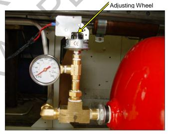
Figure 3-23 Air Pressure sensor
