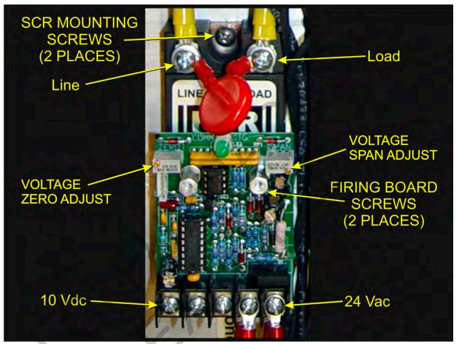
Figure 3-24 SCR installed
