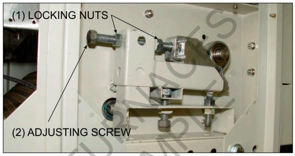
Figure 3-19 Adjust Belt Alignment
