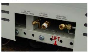
Figure 1-29 UCD Water Connections with Air Purge
