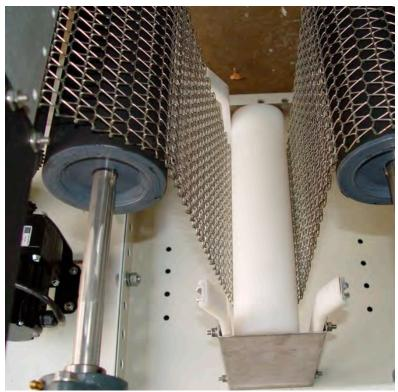
Figure 1-9 Proper Alignment of Belt Weight
