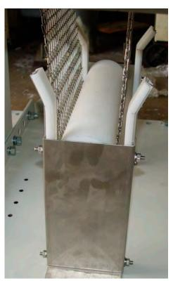
Figure 1-8 Belt Weight in Place
