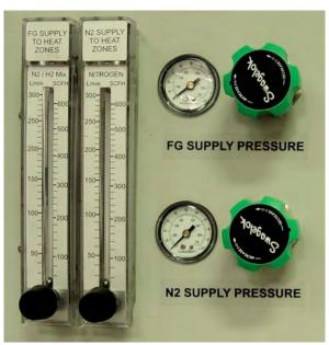
Figure 1-23 Supply Gas Mixing System
