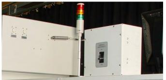
Figure 1-13 Typical Circuit Breaker Enclosure Location (option)
