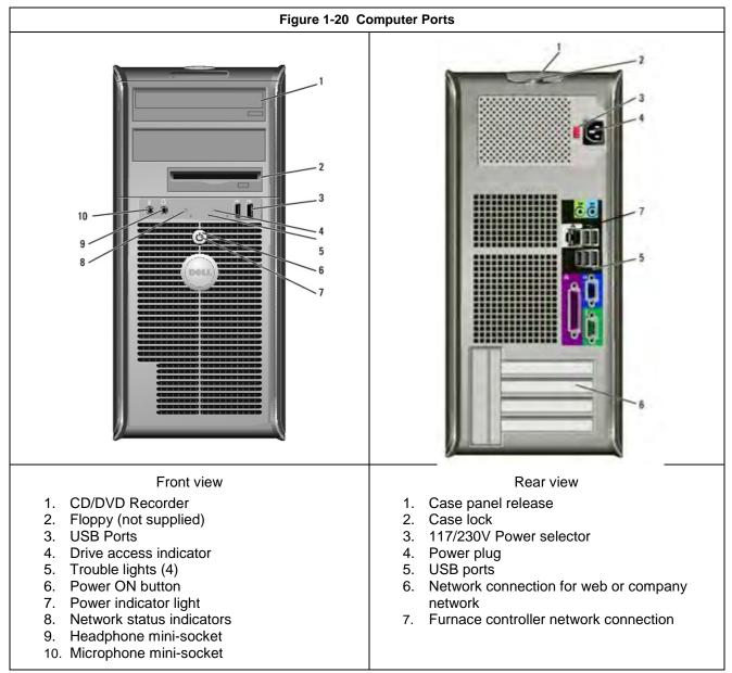
Owner may connect a network enabled 10/100/1000 Ethernet cable to the  $2^{nd}$  network port (6) on the furnace computer. Note: The motherboard Ethernet connection is reserved for the furnace controller.
