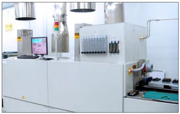
Figure 1-28 Typical Hydrogen Furnace Process Gas Exhaust Connection
