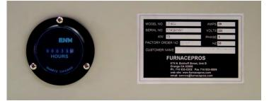
Figure 1-12 Elapsed Time Meter and Nameplate
