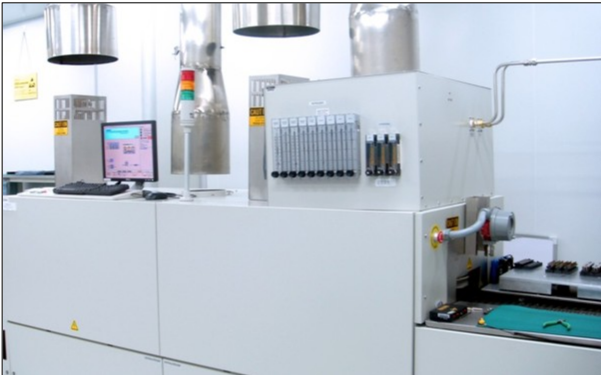
Figure 2-30 Typical Hydrogen Furnace Process Gas Exhaust Connection
