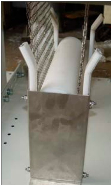
Figure 2-11 Belt Weight in Place
