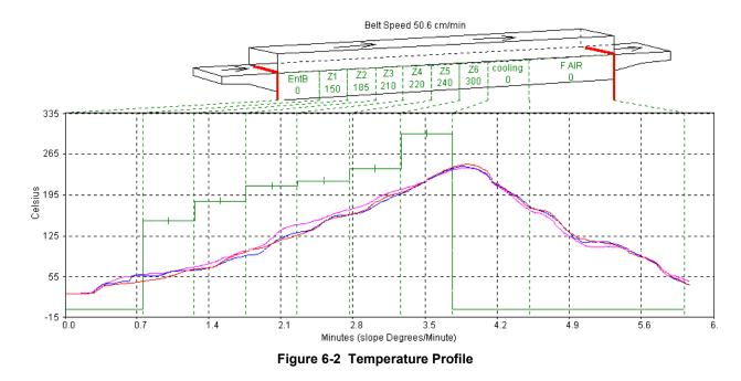
The temperature profile will be affected by the product material, mass and process gas. For example, a furnace with a controlled atmosphere cooling module installed can cool the product while in a pure nitrogen gas environment. The same temperature profile could be achieved with a forced-air cooling module, but could subject the product to a potentially hazardous oxidizing environment at elevated temperatures.
