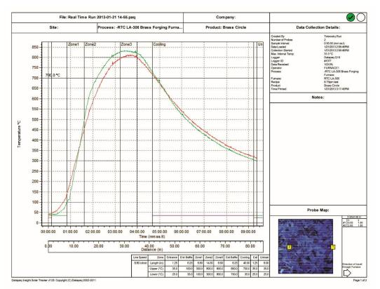
Figure 6-14 880 °C Brass Forging profile
