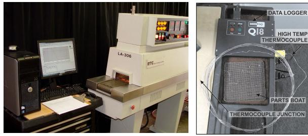
Figure 6-5 Temperature Profiling Apparatus
