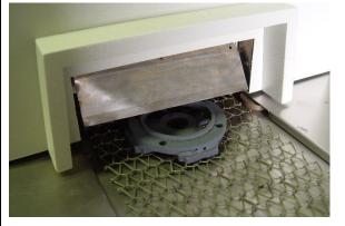
Figure 6-11 Brass forging sample exiting furnace
