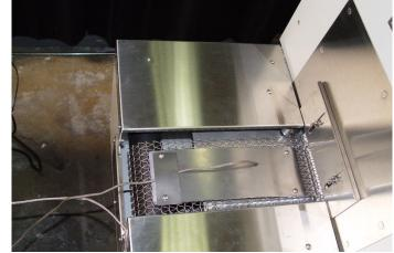
Figure 6-8 Metal Plate Sample with Wire Sheath Type K Thermocouple
