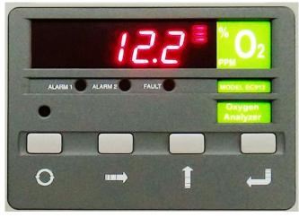
Figure 3-32 O2 Analyzer Display
