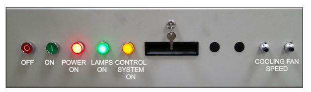
Figure 3-2 Control Console Furnace Power ON and OFF & Indicator Lights
