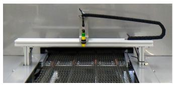
Figure 3-35 SMEMA sensor above belt
