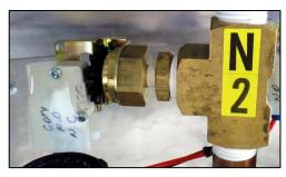
Figure 3-56 IPS Inlet Pressure Switch
