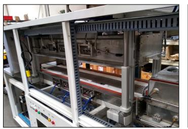
Figure 1-37 Motorized Chamber Lift
