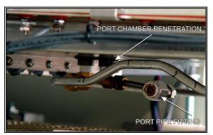
Figure 1-46 Sample Port Chamber Penetration
