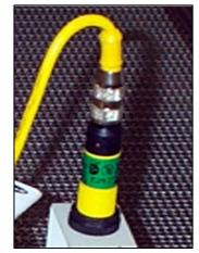
Figure 1-45 SMEMA Sensor closeup
