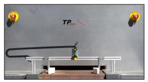
Figure 1-44 SMEMA Sensor Mount
