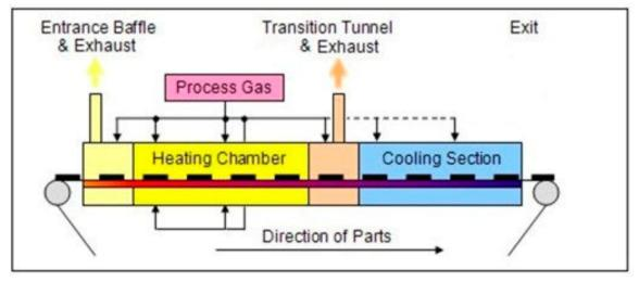
Figure 1-7 Process Sections
