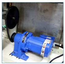
Figure 1-20 Transport Drive Motor
