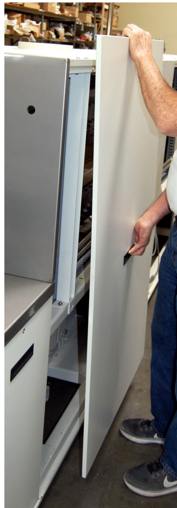
Figure 4-9 Lift panel straight up
