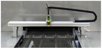
Figure 3-35 SMEMA sensor above belt
