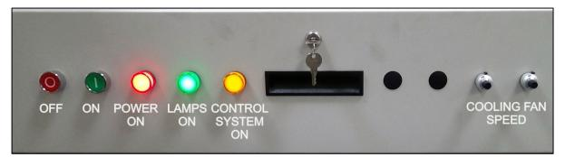
Figure 3-2 Control Console Furnace Power ON and OFF & Indicator Lights
