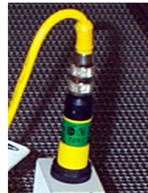
Figure 4-36 SMEMA Sensor detail
