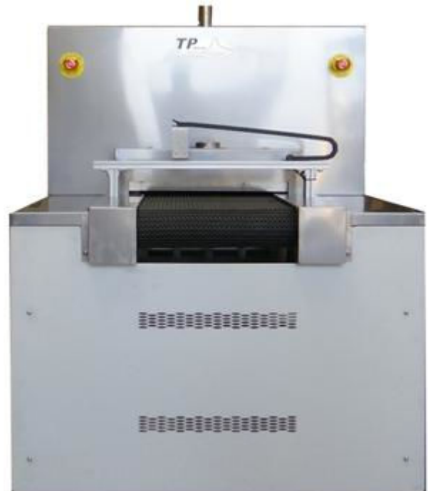
Figure 4-6 Exit Enclosure Access Panels
