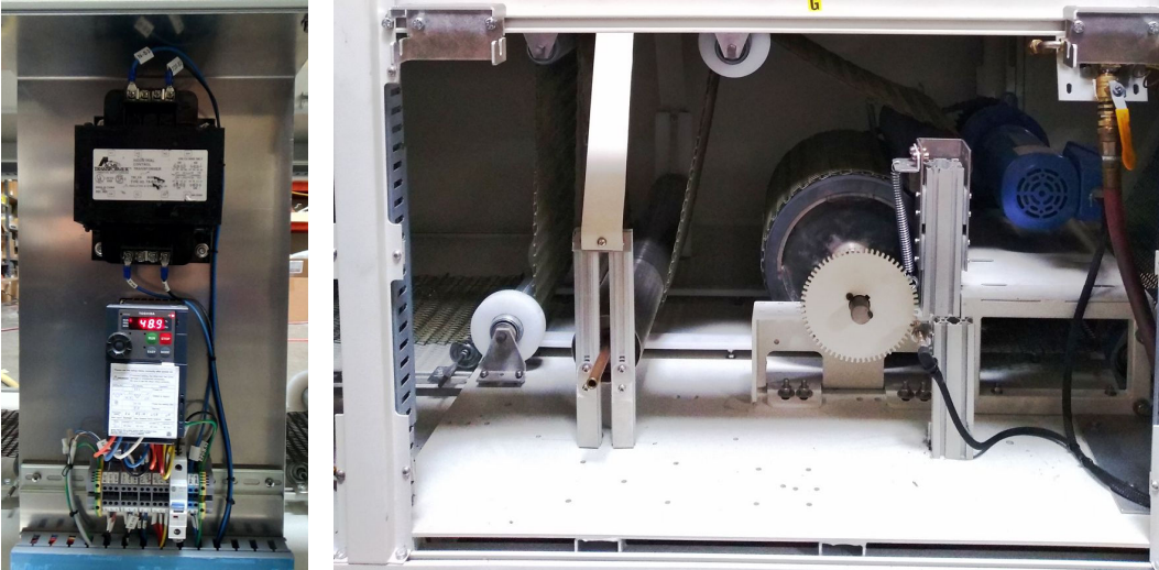
Figure 4-23 Motor Controller (L) and Drive Motor ®
