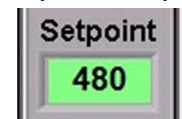
Figure 3-9 Zone Temperature setpoint
