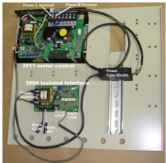
Figure 1 Motor control Panel Layout
