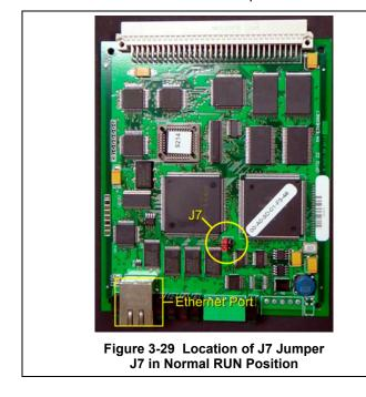
f. Move the J7 Jumper to the Module Reset Position as shown in the following pictures.
