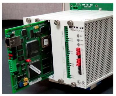
Figure 3-28 Removal of Ethernet Card
