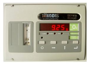
Figure 4-55 OSS Sample System Panel & Oxygen Analyzer
