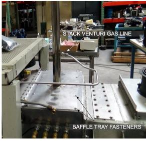
**Figure 4-38 Transition Tunnel**
