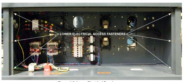
Figure 4-5 Lower Electrical Panel access
