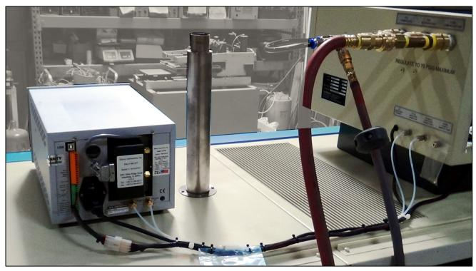
Figure 4-12 Oxygen Analyzer furnace connections
