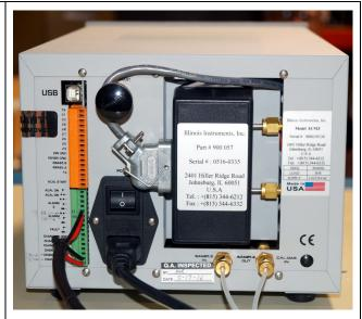
Figure 4-14 O2 Oxygen Analyzer & OSS encl-rear
