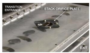
Figure 4-40 Transition Tunnel Stack Orifice Plate
