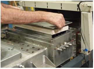
Figure 4-41 Baffle Tray in Transition Tunnel
