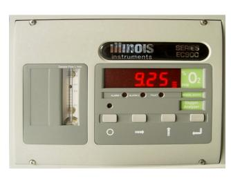
Figure 4-13 OSS & O2 Analyzer-front view
