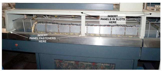
Figure 4-4 Upper Access Panel Installation
