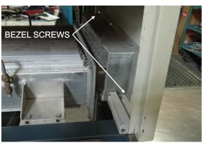
Figure 4-35 Bezel fasteners
