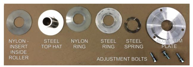
Figure 4-20 Clutch Components
