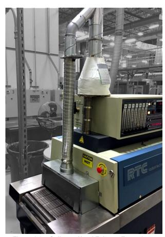
Figure 2-34 Collector Hood Exhaust Example
