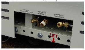
Figure 2-44 UCD Water Connections and Air Purge (Reservoir option only)
