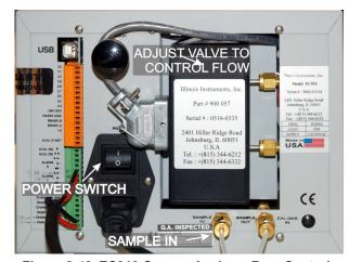
Figure 2-42 EC913 Oxygen Analyzer Rear Controls
