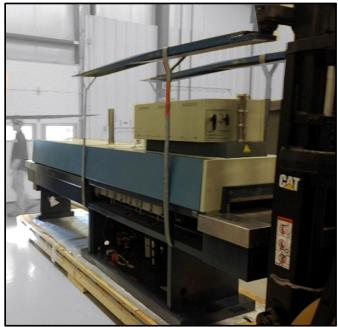
Figure 2-4 Lift Furnace with panel removed. Two-pedestal models may require the middle lift point closer to exit.
