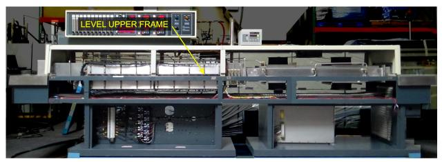
Figure 2-9 CU-915 (1984-6) Furnace Front View with panels removed.
