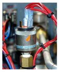
Figure 2-46 Pressure Switch
