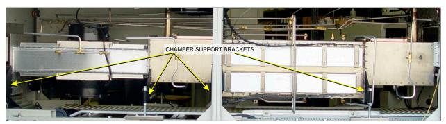
Figure 2-13 Location of Support Brackets on post-2000 model furnaces
