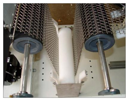
Figure 2-19 Proper Alignment of Belt Weight in guide
