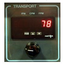
Vary the conveyor speed from minimum (4 ipm) to maximum (75 ipm) using the TRANSPORT panel BELT SPEED knob.
