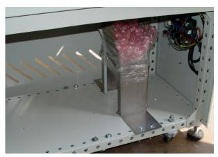
Figure 2-17 Belt Weight in guide with packing
