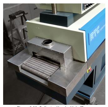
Figure 2-33 Collector Hood with baffle
