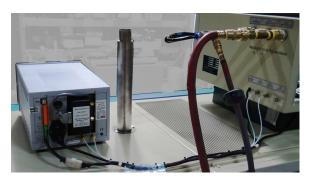
Figure 2-39 Locate oxygen analyzer next to OSS
