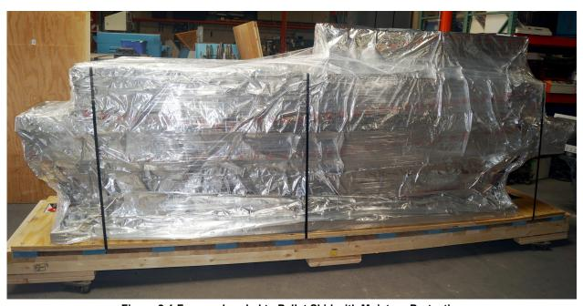
Figure 2-1 Furnace banded to Pallet Skid with Moisture Protection
