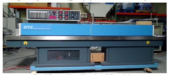
Figure 2-2 Furnace on blue steel frame shown with Oxygen Analyzer
