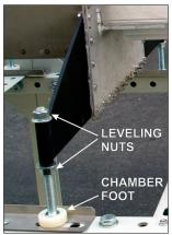
Figure 2-11 Chamber Support Bracket
